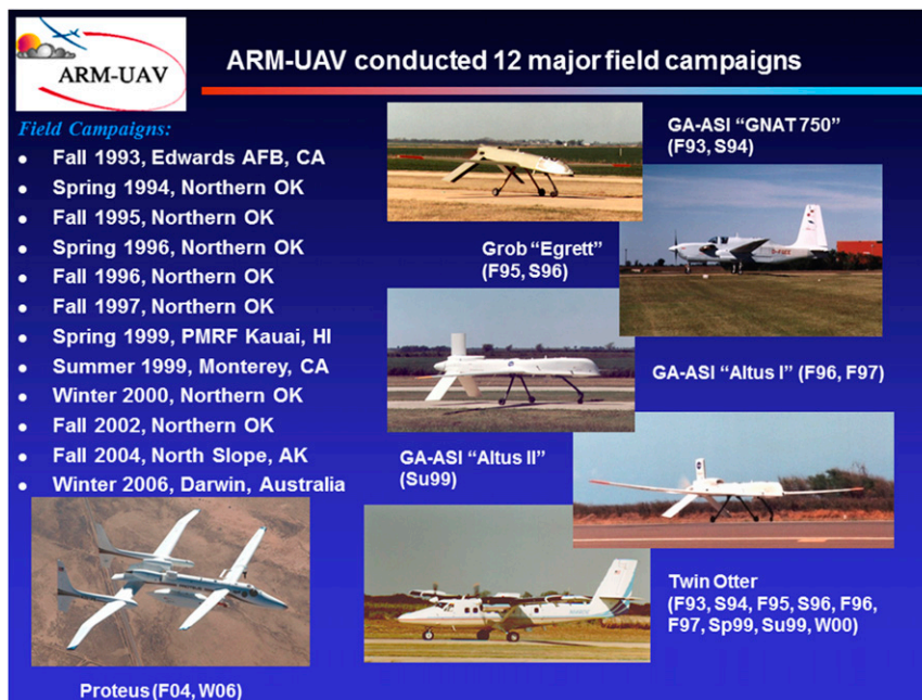
FIG. 10-1. Platforms used and field campaigns conducted by the ARM-UAV program. Seasons are denoted as follows: summer (S), spring (Sp), fall (F), winter (W), and summer (Su). Years are given as follows: 9x and 0x denote 199x and 200x, respectively.
