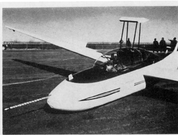
FIG. 3. Photograph of the disdrometer mounted on a 75 cm long boom on "The Explorer" sailplane.
