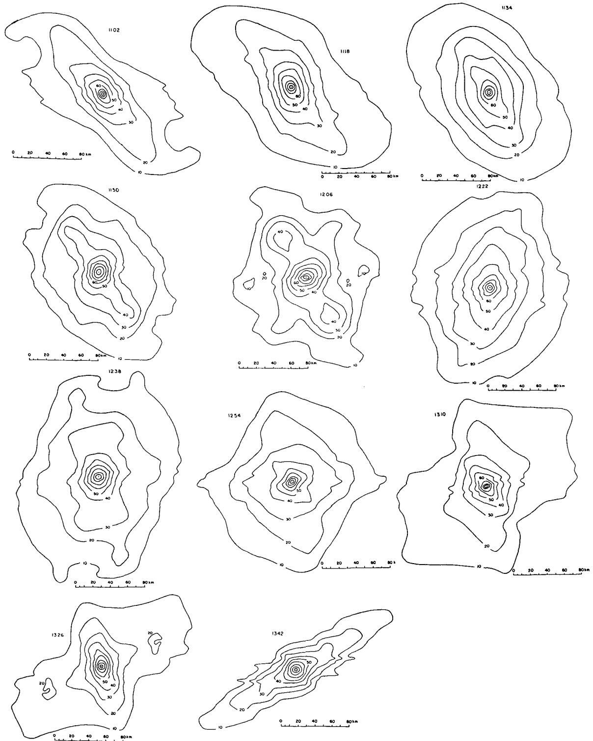
FIG. 11. Normalized space ACF's at 16-min intervals covering the period 1102-1342 of the storm of 16 September 1969.
