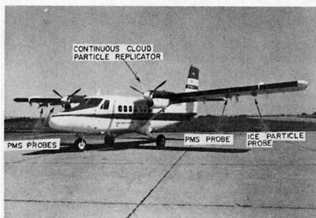
FIG. 1b. DHC-6 Twin Otter aircraft instrumented for cloud microphysical measurements.
