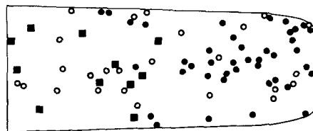
FIG. 3. Map of the filter surface drawn on the basis of serial photographs of the ice nuclei active after 2 min (black squares), 4 min (black circles) and 8 min (open circles). The filter sampled urban air.
