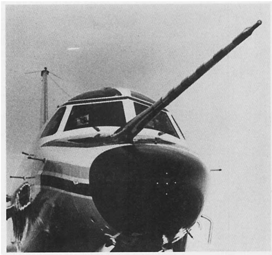
FIG. 4. Photograph of NCAR Sabreliner Model 65 showing nose boom with 858 pressure sensor and pressure holes in radome.
