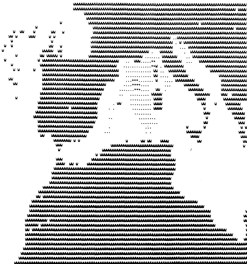
FIG. 5. The figure shows the METEOSAT picture of 27 July at 1130 UTC, over the Mediterranean Sea. Every B2 pixel has been displayed, with different label according to its digital count. The W label corresponds to a digital count larger than 60, and no label corresponds to a digital count smaller than 20 (clear sky). The coasts are well recognizable and no cloud structure appear with sharp edges and large reflectances. The reflectance behavior in the middle of the picture indicates the large and smooth saharan dust cloud.
