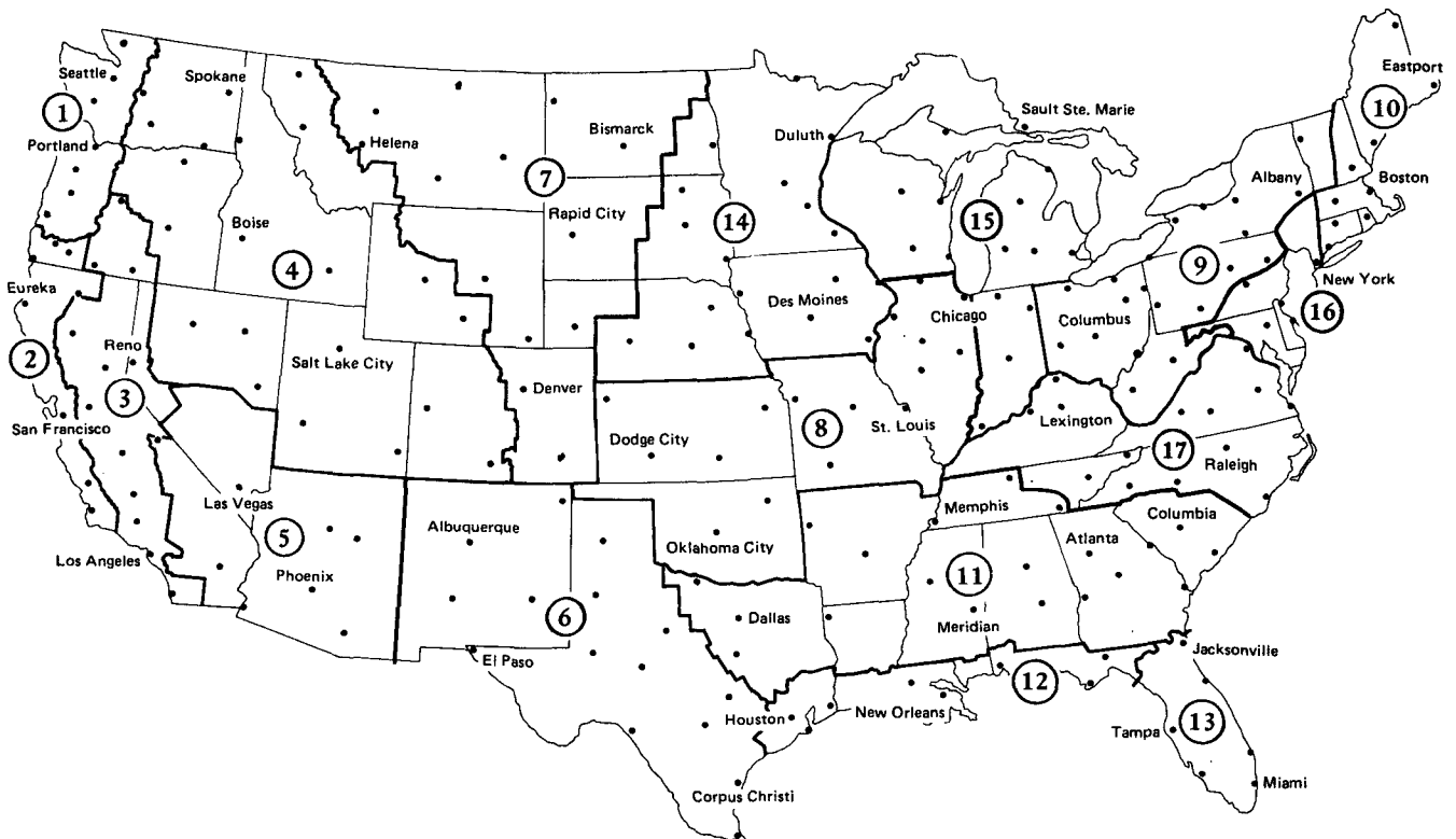
FIG. 4. Rate areas and recording raingage stations used to compute rate area values.
