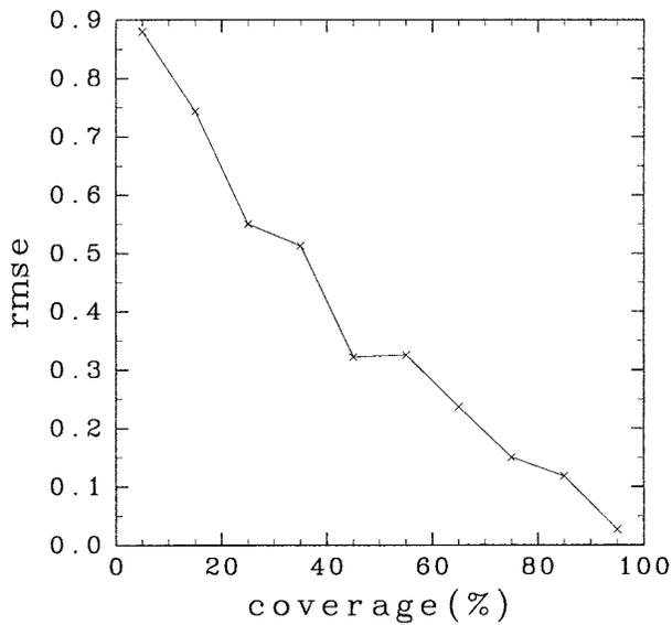
FIG. 7. Root-mean-square error ( $\text{mm h}^{-1}$ ) between rain rate averaged in the entire area and estimated by the threshold method in the observed area. The X axis is the ratio of observed area to whole area. This is the case of region B ( $5^\circ \times 5^\circ$ ).
