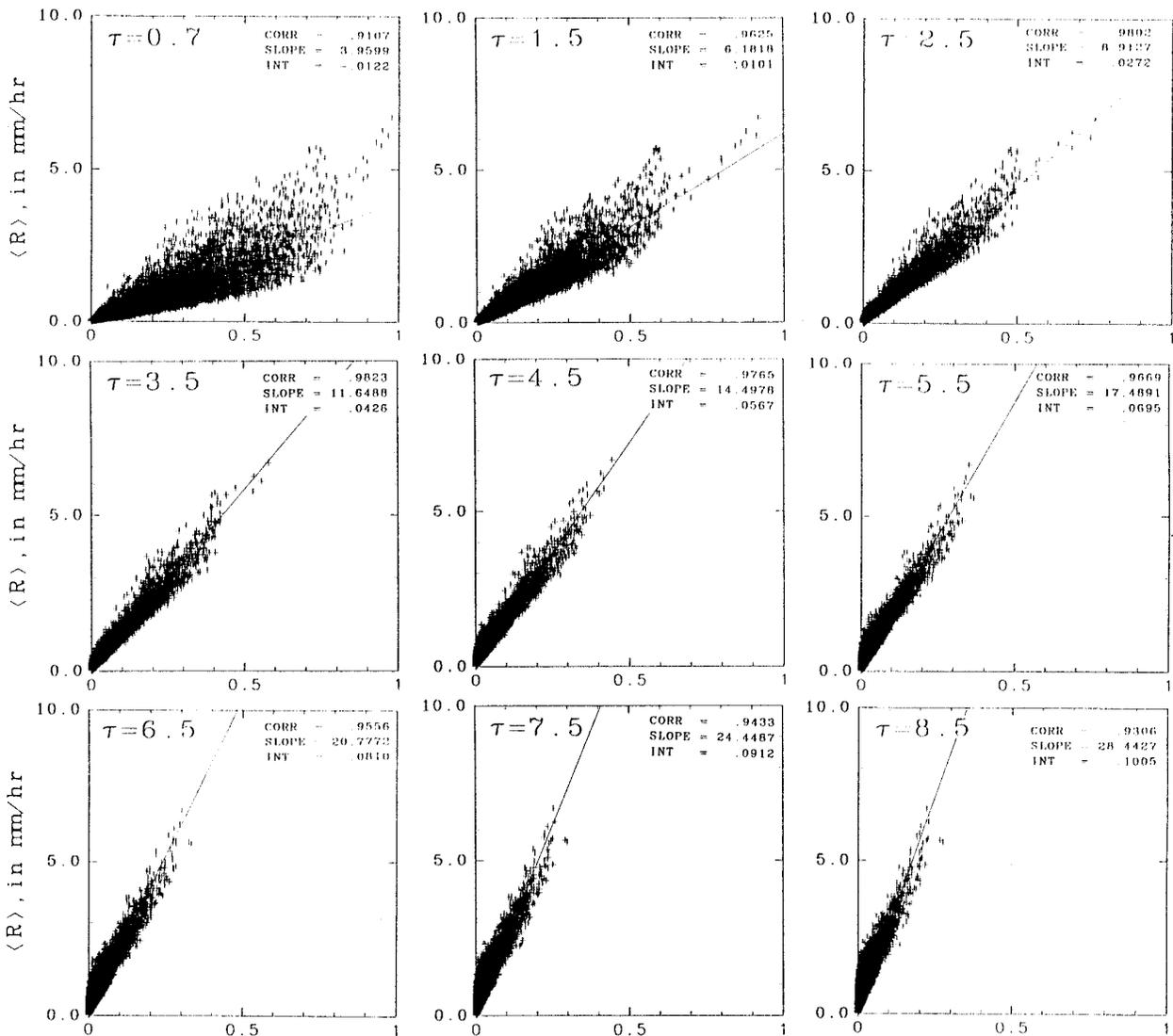
FIG. 4. Area-average rain rate versus fractional coverage of rain rates exceeding  $\tau$  mm h<sup>-1</sup> (0.7–14.5 mm h<sup>-1</sup>) over a  $5^\circ \times 5^\circ$  subset of the radar-AMeDAS hourly rain rates, from March 1988 to September 1991, region B.
