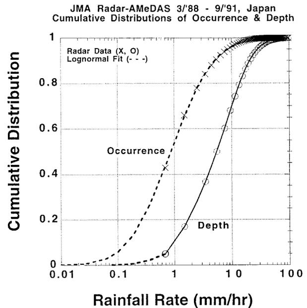
FIG. 3. Normalized distributions of the cumulative rainfall by depth and occurrence. The percentage of rain rates observed below  $1 \text{ mm h}^{-1}$  is 53% in occurrence and only about 12% in depth.
