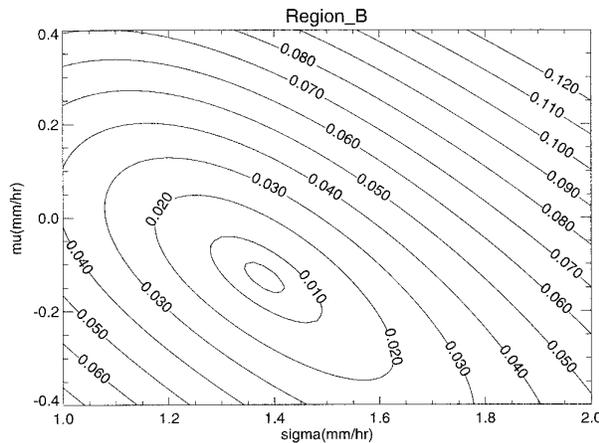
FIG. 2. The rms difference between CDF from the data and a model (lognormal) CDF in  $\mu$  and  $\sigma$  space. For region B, the best fit is found for  $\mu = -0.13$  and  $\sigma = 1.38$ .
