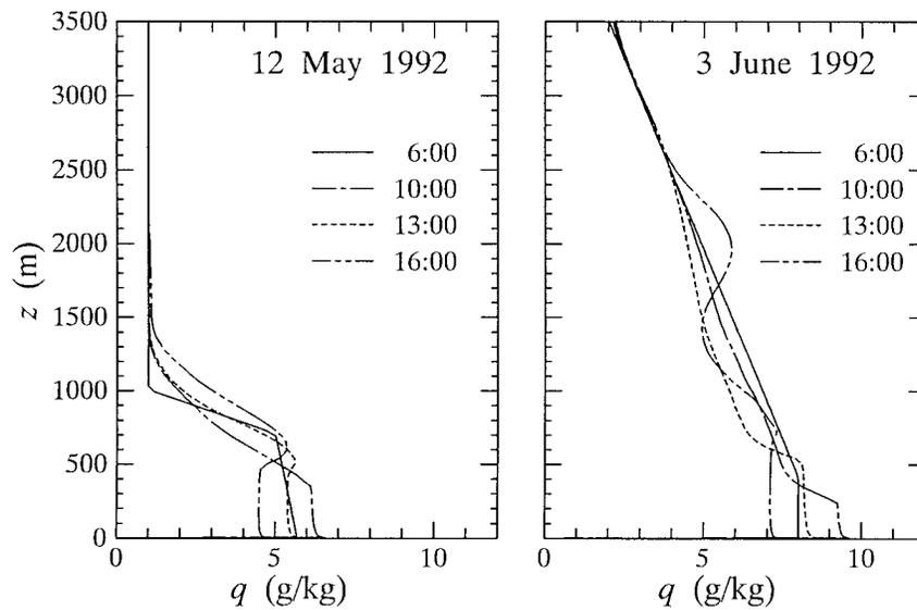
FIG. 12. Daily variations of the calculated specific humidity profiles at a model site 5 km from the center of the valley on 12 May (left) and 3 June 1992 (right). The times are indicated in the figure legends.
