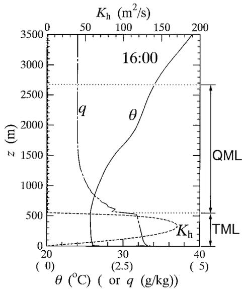
FIG. 4. The coefficient of vertical turbulence for heat  $K_h$  (dotted line) calculated by the numerical model at 1600 LT 12 May 1992, together with the simultaneous potential temperature (solid line) and specific humidity (chain line) profiles at the center of the valley for  $U = 0 \text{ m s}^{-1}$  (TML: turbulent mixed layer, QML: quasi-mixed layer).
