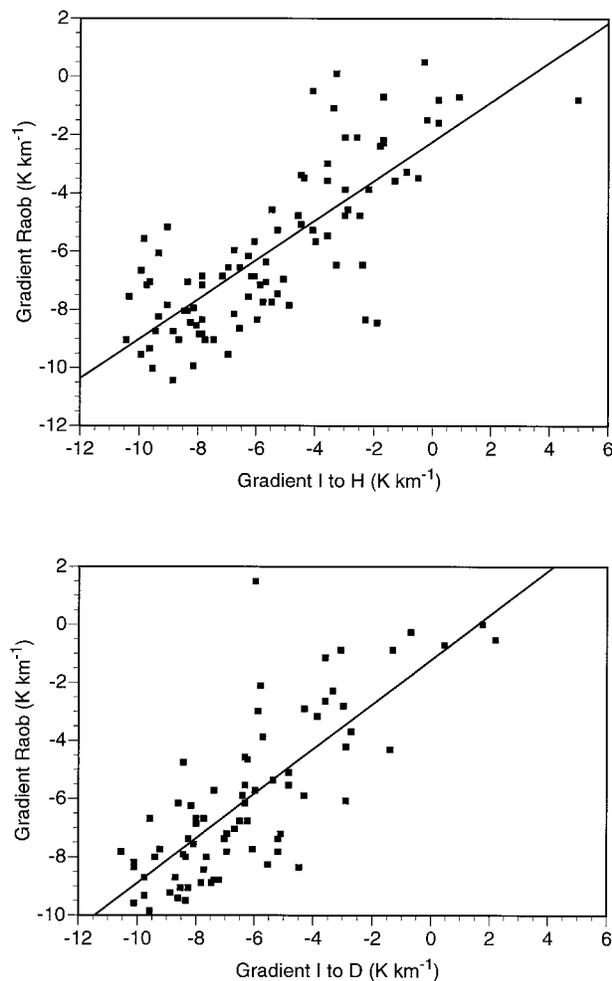
FIG. 4. Scatter diagrams of temperature gradients calculated from surface stations ( $x$  axis) and from soundings at the corresponding heights ( $y$  axis). Top panel: gradients between heights of Indian Garden and Hopi Point (correlation coefficient  $r = 0.78$ ). Bottom panel: gradients between heights of Indian Garden and Desert View ( $r = 0.78$ ).
