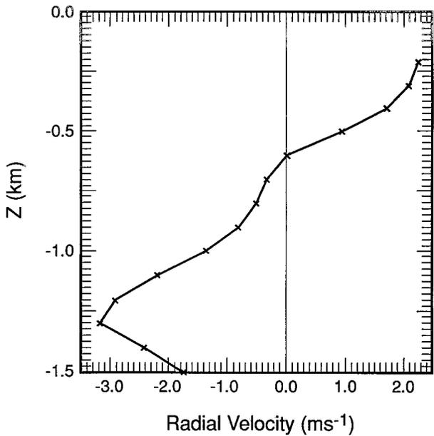
FIG. 11. Vertical profile of mean  $u_r$ , showing peak speeds of  $3.1 \text{ m s}^{-1}$  in the jet of down-canyon flow at  $z = -1.3 \text{ km}$ , i.e., below the south rim. The wind gradually decreased in speed with height and switched to southerly flow above  $-0.6 \text{ km}$ . The profile, centered at  $x = 1.0 \text{ km}$  and  $y = 8.6 \text{ km}$ , was from the volume shown in Fig. 10.
