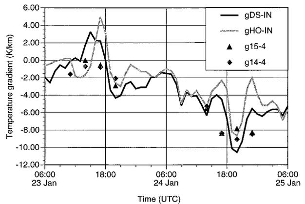
FIG. 8. Hourly values of the stability as measured by surface-station temperature data for 23–25 January 1990 UTC. Also plotted are values from airsonde measurements ( $\blacktriangle$  and  $\blacklozenge$ ). Temperature gradients: gDS-IN calculated between Desert View and Indian Garden surface stations, gHO-IN between Hopi Point and Indian Garden, g15-4 between the 1500 m and 400 m AGL sounding levels, and g14-4 between 1400 m and 400 m AGL sounding levels.
