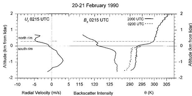
FIG. 6. Vertical profiles from near the canyon bottom to above the south rim showing the radial velocity ( $u_r$ ,  $\text{m s}^{-1}$ ) and backscatter intensity ( $B_s$  in dB), from a Doppler lidar scan on 21 February 1990 at 0215 UTC. Also shown are potential temperature profiles ( $\theta$  in K), from the Phantom Ranch airsonde at 2000 UTC on 20 February (solid line) and from the Phantom Ranch tethersonde at 0200 UTC on 21 February 1990 (dashed line).
