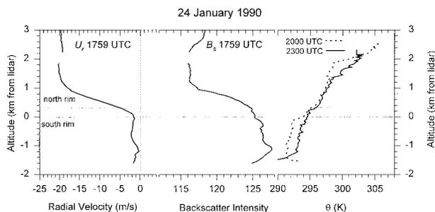
FIG. 7. Vertical profiles of the radial velocity ( $u_r$ ,  $\text{m s}^{-1}$ ) and backscatter intensity ( $B_s$  in dB), as in Fig. 6, except from a Doppler lidar scan on 24 January 1990 at 1759 UTC. Also shown are potential temperature profiles ( $\theta$  in K), from the Phantom Ranch airsonde at 2000 UTC (dashed line) and at 2300 UTC (solid line).
