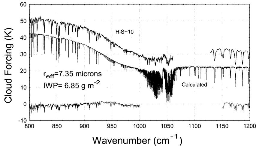
FIG. 7. Cloud forcing as a function of wavenumber for an HIS observed spectrum during the SUCCESS experiment (cloud 998) and results from a DISORT calculation with an effective radius of  $7.35 \mu\text{m}$  and an IWP of  $6.85 \text{ g m}^{-2}$ . Here, 10 K is added to the HIS spectrum (top) for clearer distinction from the DISORT calculation (middle). The bottom spectrum is the difference between the two at wavenumbers of HIS resolution used in the rms calculation.
