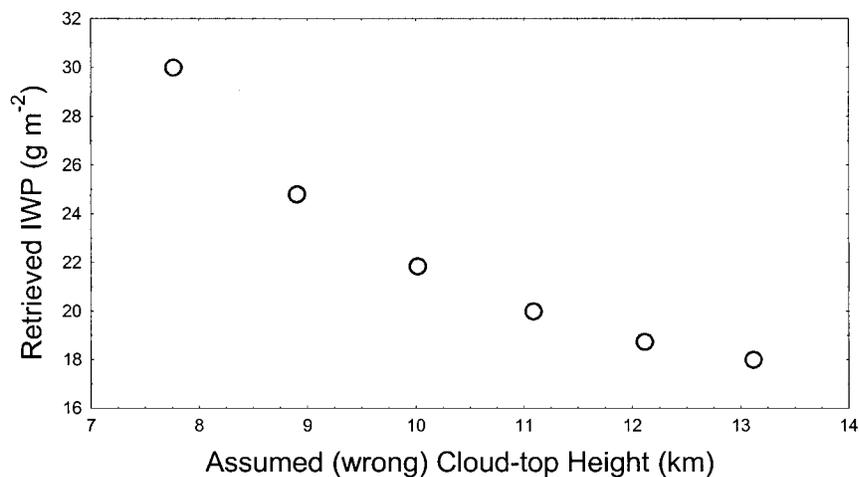
FIG. 3. Errors in retrieved IWP if the cloud-top altitude is assigned incorrectly during the retrieval. The ice cloud has an IWP of  $20 \text{ g m}^{-2}$ , an effective radius of  $30 \mu\text{m}$ , and exists between 11.1 and 10.0 km.
