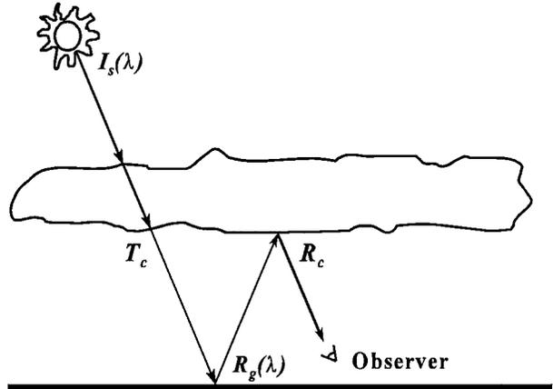
FIG. 1. Schematic representing the geometry of the nonabsorbing ground reflection problem. Here,  $T_c$  and  $R_c$  are the transmissivity and reflectivity of the cloud,  $R_g$  is the spectral reflectance of the ground, and  $I_s$  is the spectral solar radiance.
