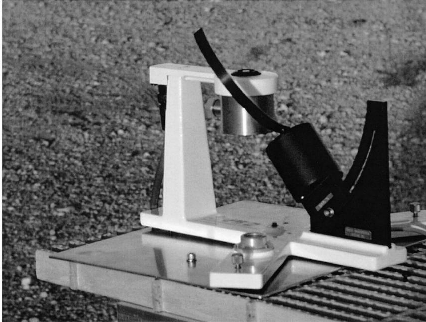
FIG. 1. The Multifilter Rotating Shadowband Radiometer.
