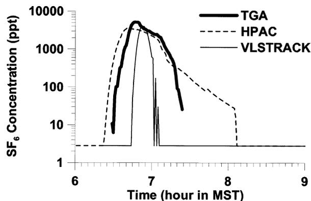
FIG. 5. Time series of 60-s-average  $\text{SF}_6$  concentrations observed by the TGA (thick solid) and predicted by HPAC (dashed) and VLSTRACK (thin solid) at the east end of the middle sampling line ( $\sim 5$  km from the source) for OLAD trial 5. A lower concentration threshold of 3 ppt was used.
