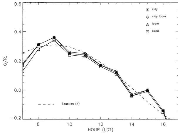
FIG. 2. Time series of simulated  $G/R_n$  for the 11 soil types (Clapp and Hornberger 1978), using an initial upper-volumetric soil moisture of 0.40 and average atmospheric forcing from Monsoon '90. Included are estimations from (4), a constant ratio, and that of Cellier et al. (1996).
