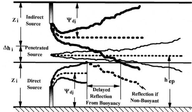
FIG. 3. AERMOD’s three-plume treatment of the CBL.
