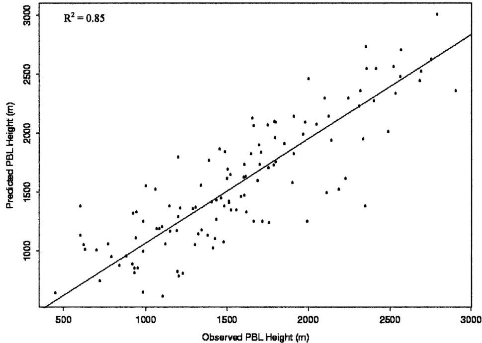
FIG. 9. Observed PBL height  $h$  vs that predicted using the trend surface in Fig. 7 and 132 daily observations of stability, soil water content, and 2-m potential temperature change.
