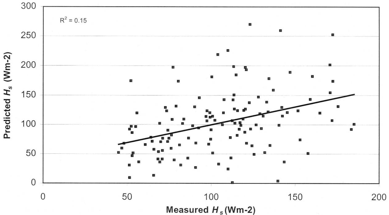
FIG. 5. Measured surface sensible heat flux vs the flux estimated using closure of the conservation equation and prescribing entrainment as 48% of the surface flux ( $A_R = 0.48$ ).
