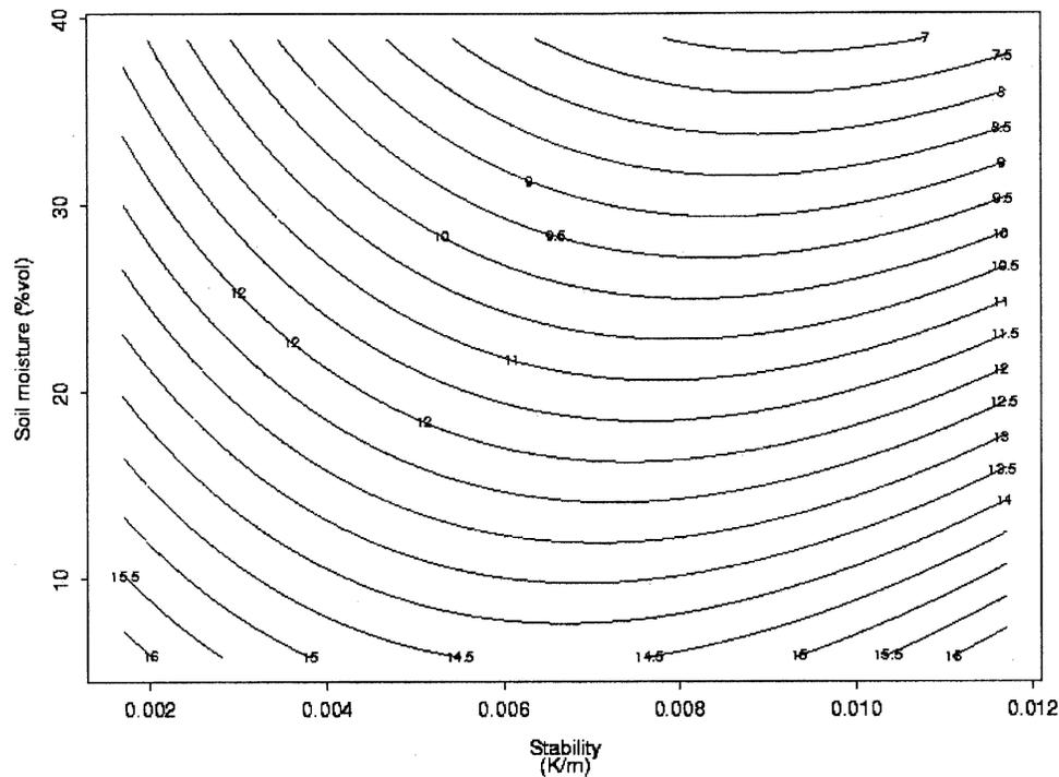
$$\Delta\theta_{2m} = 10.72 - 0.96\gamma_{ml} - 3.53\gamma_{ml}^2 + 1.94w - 1.07w\gamma_{ml} - 0.16w^2$$
