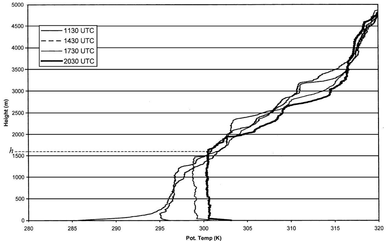
FIG. 1. Profiles of potential temperature taken from radiosonde soundings at the Lamont, OK, ARM-SGP site on 5 Jun 1997. The launch times correspond to 0630, 0930, 1330, and 1630 local time. Also labeled is the maximum height of the PBL ( $h$ ).
