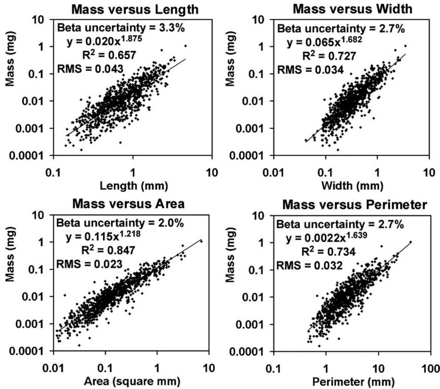
FIG. 3. Log-log plots of mass vs each of the various individual size parameters  $L$ ,  $W$ ,  $A$ , and  $P$ . The least squares regression line, equation, and correlation coefficient squared are shown along with the rms error. The latter is calculated from the values themselves, not from their logarithms.
