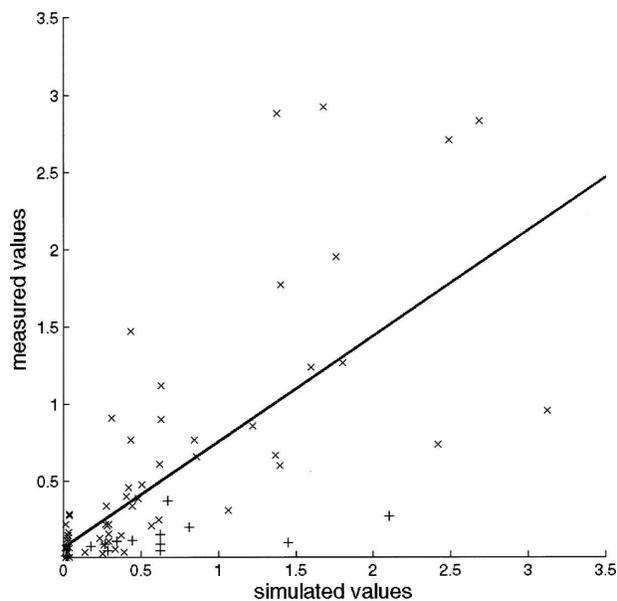
FIG. 6. Scatterplot of simulated mean concentrations of B(a)P ( $\text{ng m}^{-3}$ ) against measured values. The plus signs denote weekly means from Bornhoeved ( $r = 0.75$ ), and the times signs denote 2-day means from Radebeul ( $r = 0.58$ ).
