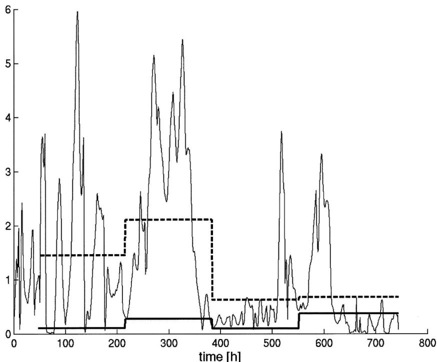
FIG. 5. Comparison of simulated hourly concentrations ( $\text{ng m}^{-3}$ ; thin line) with the measured weekly mean concentration (thick gray line) of April 2000 at Bornhoeved. The dashed line displays weekly means calculated from simulations.
