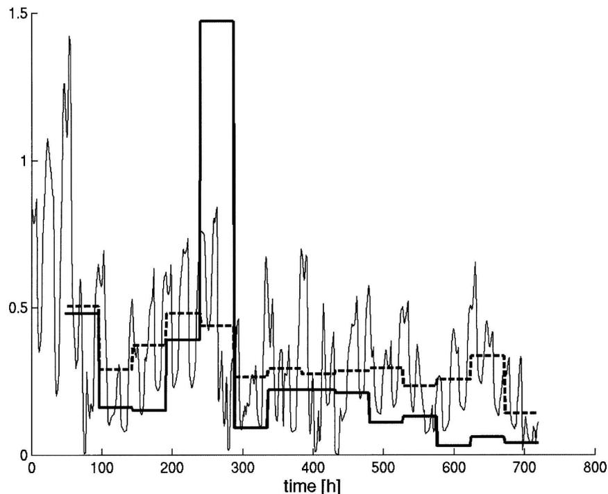
FIG. 7. Comparison of simulated hourly concentrations ( $\text{ng m}^{-3}$ ; thin line) with the measured 2-day mean concentrations (thick gray line) of April 2000 at Radebeul. The dashed line displays 2-day means calculated from simulations.
