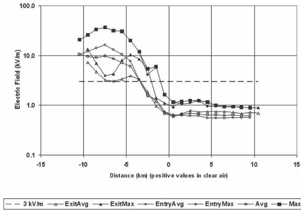
FIG. 4. Electric-field magnitude as a function of distance from the edge of anvil clouds in ABFM-II having a maximum field magnitude of at least  $3 \text{ kV m}^{-1}$ . The maximum and average values are shown separately for passes entering cloud and exiting cloud. The hazard threshold of  $3 \text{ kV m}^{-1}$  is shown by a horizontal dashed line. The cloud boundary is at the midpoint of the chart (distance = 0) with cloud on the left and clear air on the right.
