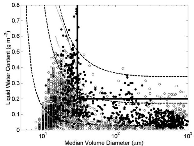
FIG. 2. Comparison of three of the four icing envelopes shown in Fig. 1 with 2444 SLD icing environments observed at 3-km resolution and reported by Cober and Isaac (2012). Data points for which the  $\text{LWC} \times 80\text{VD}$  values are between 10 and  $100\text{ g m}^{-3}\mu\text{m}$ , corresponding to the envelopes of Ashenden and Marwitz (1998), are shown as filled circles.
