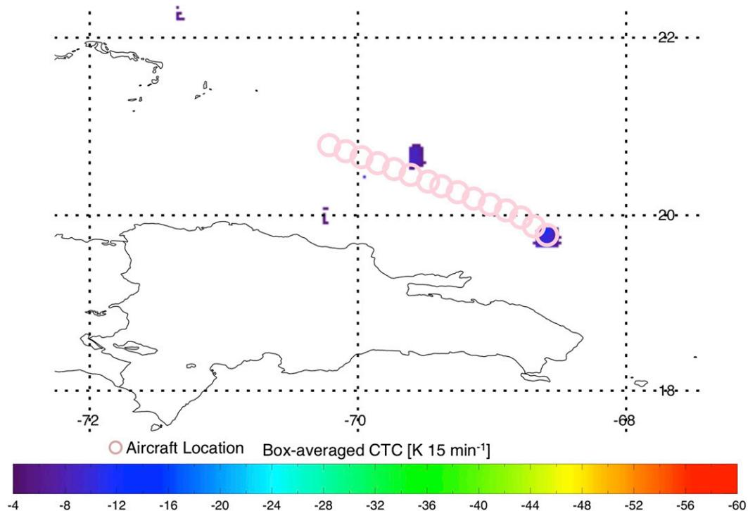
FIG. 1. CTC and Continental Airlines flight 128 track at 0802 UTC 3 Aug 2009. The plotted track is within  $\pm 7$  min of the satellite scan time. Note the flight track over the colored CTC just north of Hispaniola's eastern point. The timing of this occurrence corresponds to the time that the Boeing 767-200 aircraft experienced turbulence.
