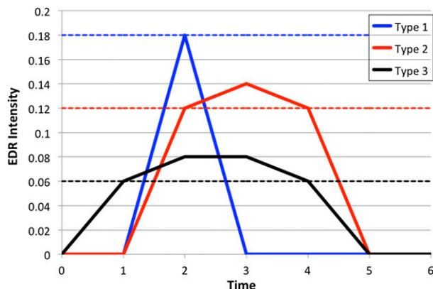
FIG. 2. Schematic illustrating the Delta Airlines EDR reporting triggering logic. Blue represents a type-1 report in which an EDR value greater than or equal to 0.18 is experienced. Red represents a type-2 report in which an EDR value greater than or equal to 0.12 is experienced for at least 3 out of the last 6 min. Black represents a type-3 report in which an EDR value greater than or equal to 0.06 is experienced for 4 out of the last 6 min.
