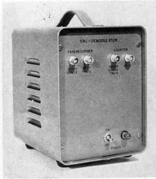
FIG. 6. The demodulator used with the HRPS. This connects the GMD-1B ground tracker with a frequency-counter and printer for pressure data and connects the GMD to the TMQ-5 for the other standard meteorological data.
