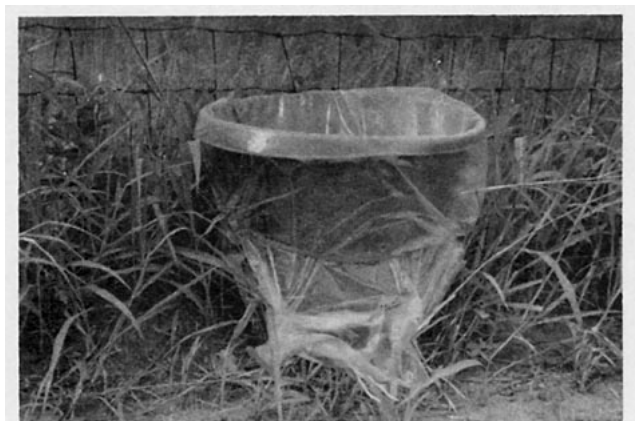
FIG. 5. Samplers distributed by the mobile units are plastic yard baskets of 20-inch diameter at the mouth, lined with polyethylene bags. The liner is held by a rubber band which also serves to support the unit against a roadside fence. The samplers are pre-inoculated with 50 ml of 6N HCl to assure acid solution of all tracer indium in the collected sample.
