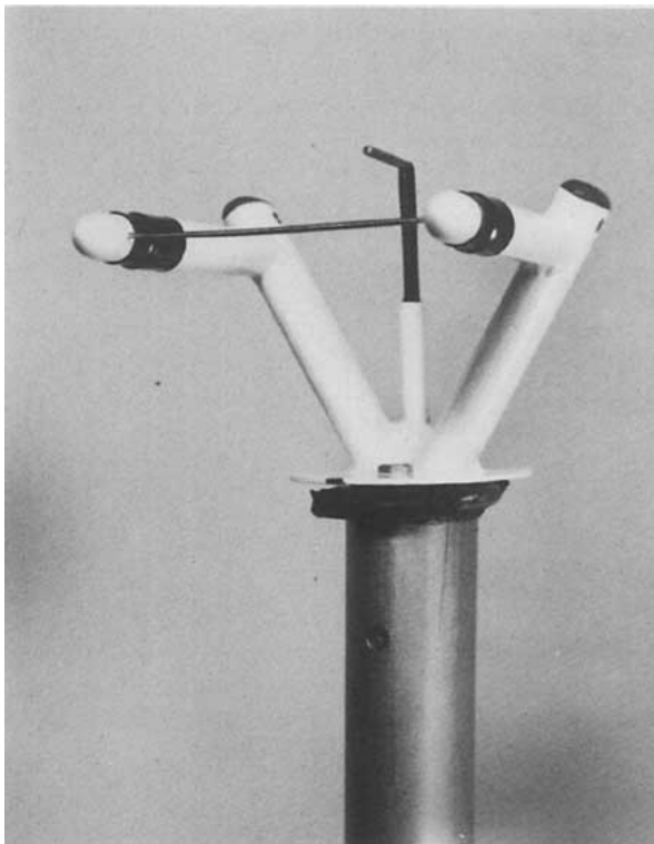
FIG. 2. Details of the retractable hot-wire probe and pitot-static tube.
