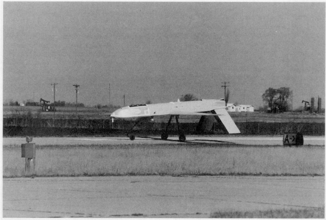
FIG. 1. Photo of the UAV with radiometers installed. One solar broadband, one infrared broadband, and one TDDR are in the top, looking upward. Another solar-infrared broadband pair is installed in the bottom, looking downward. The landing gear is retracted for cruise and ascents and extended for descents and landing.
