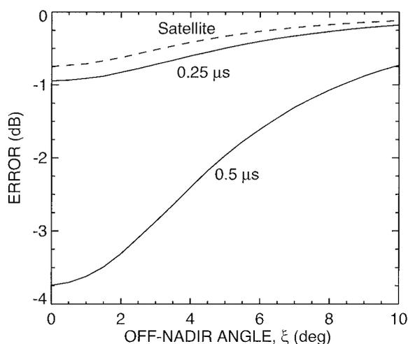
FIG. 11. Computed error as a function of the antenna angle off-nadir ( $\xi$ ) using the EDOP system parameters. Errors are shown for gate spacings of  $0.5 \mu\text{s}$  (current configuration) and  $0.25 \mu\text{s}$ . The dashed line is for a radar such as will be flown on the NASA TRMM satellite.
