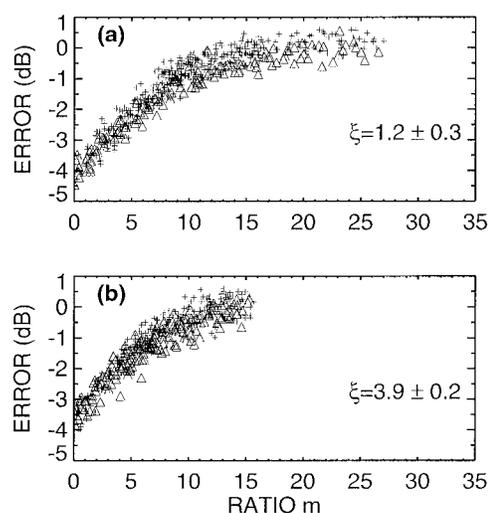
FIG. 12. (a) Scatterplot of  $m$  versus estimated error for the data shown in Fig. 4. The mean incidence angle is  $1.2^\circ$ . (b) Example of  $m$  for a case at 1757 UTC 11 January 1995, where the mean incidence angle is  $3.9^\circ$ . In both panels, the contributions are shown for  $m_d$  (+) and  $m_u$  ( $\Delta$ ).
