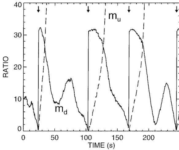
FIG. 6. Ratio of the signal in the gates around the peak surface echo for the data in Fig. 4. Ratio  $m_d$  is the solid line and  $m_u$  is the dashed line. The arrows indicate times at which the peak surface echo moved from one gate to the next.
