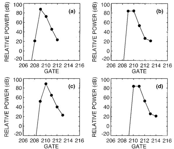
FIG. 5. Range profiles of the surface echo on 28 August 1995 at selected times from Fig. 4: (a) 70 s, (b) 103 s, (c) 130 s, and (d) 168 s. The gate spacing is 75 m.
