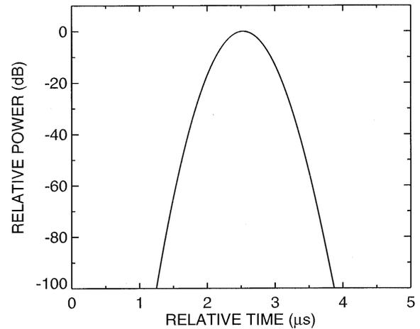
FIG. 1. Example of the received surface echo for nadir incidence ( $\xi = 0$ ).
