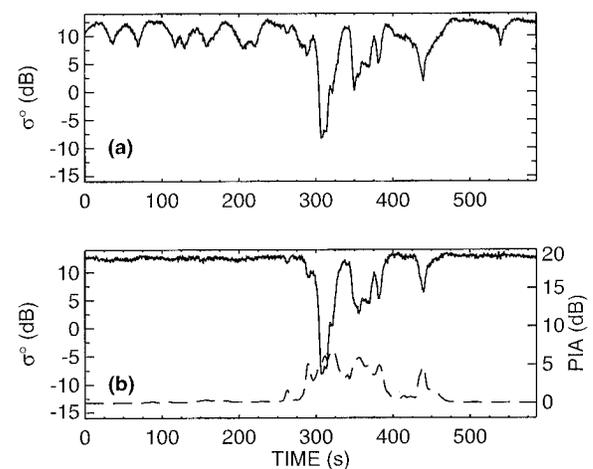
FIG. 10. (a) Observed surface cross section under a storm at 2203 UTC 28 August 1995. The along-track distance is 124 km. (b) The  $\sigma^o$  corrected using the ratio method described in the text. The remaining deviations (260–470 s) are a result of attenuation by rain along the propagation path. An estimate of the path-integrated attenuation (PIA) from the observed precipitation reflectivity factor is shown by the dashed line.
