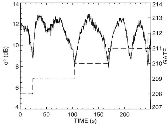
FIG. 4. Normalized surface cross section  $\sigma^o$  (solid line) observed at 2200 UTC 28 August 1995 at near-nadir incidence in a cloud-free region. The dashed line shows the range gate number where the surface peak echo is found. The dashed line indicates the increasing range to the surface as the aircraft changes altitude. The along-track distance is 52 km.
