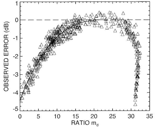
FIG. 7. Scatterplot of the ratio  $m_d$  versus estimated error from the baseline cross section for the data in Fig. 4. The solid line is the best-fit curve obtained from a regression analysis.
