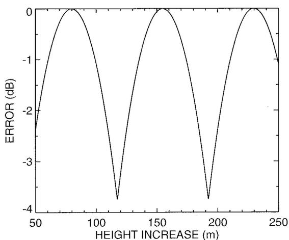
FIG. 2. The surface echo from Fig. 1 sampled with a gate spacing of  $0.5 \mu\text{s}$  at nadir incidence. Aircraft altitude increases linearly.
