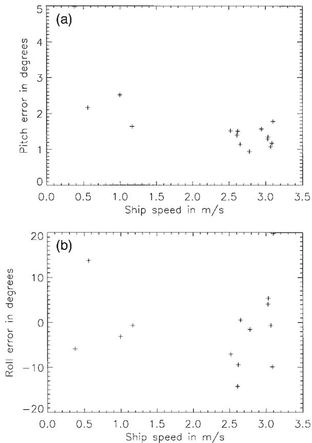
FIG. 3. (a) Pitch and (b) roll errors, respectively, as a function of ship speed based on a correction for each 1.0-min sample over the flat portion of the topography.
