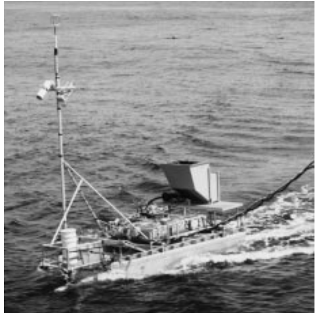
FIG. 3. The R/P LADAS catamaran. The sonic anemometer is mounted on the mast above the starboard pontoon. The Honeywell AMU was located in one of the splash-proof containers near the center of the catamaran.
