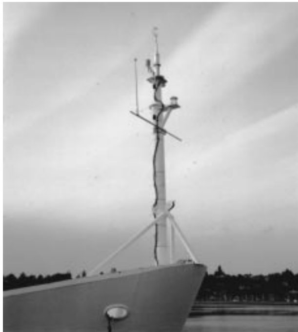
FIG. 4. The Direct Covariance Flux System used aboard the R/Vs Iselin and Wecoma . The anemometer is mounted directly above the metal canister that houses the MotionPAK AMU sensors. The sensor mounted horizontally below the canister is an Ophir infrared hygrometer. The antenna for the GPS receiver integrated into the system is visible on the horizontal crosspiece.
