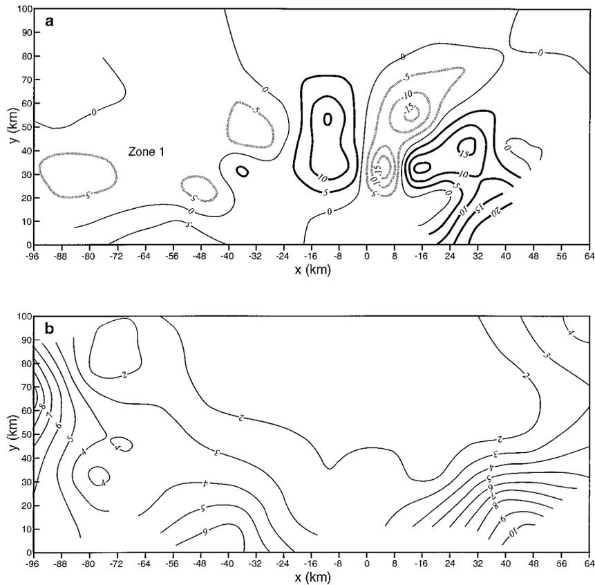
FIG. 3. The VVP results computed from Doppler velocity data at 0630 UTC for (a) divergence field contoured every  $5 \times 10^{-4} \text{ s}^{-1}$ ; (b) standard error of divergence estimate,  $\sigma_d$ , contoured every  $10^{-4} \text{ s}^{-1}$ ; (c) horizontal deformation,  $(u_x + v_y)$ , contoured every  $2 \times 10^{-4} \text{ s}^{-1}$ ; and (d) vertical wind shear,  $(u_z^2 + v_z^2)^{1/2}$ , contoured every  $2 \times 10^{-3} \text{ s}^{-1}$ .
