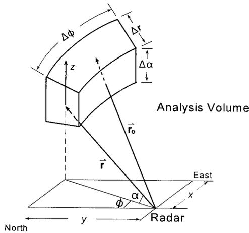
FIG. 1. Geometry of the analysis volume for the velocity volume processing technique. The  $r$ ,  $\phi$ , and  $\alpha$  are the radar detecting range, azimuth, and elevation angles, respectively. The range vector  $\mathbf{r}_o$  is directed to the center of the analysis volume from the radar.
