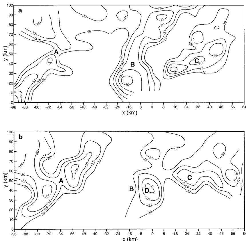
FIG. 2. Radar reflectivity PPI (dBZ) at an elevation angle of  $1.5^\circ$  observed at (a) 0630 UTC and (b) 0700 UTC 19 August 1992. The  $x$  axis points eastward with the radar sited at (0, 0). The radar echo intensity is contoured every 5 dBZ.
