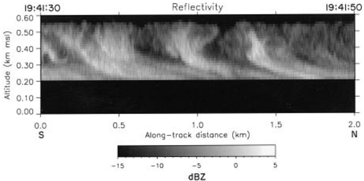
FIG. 9. South-north reflectivity cross section. The curvature of the high-reflectivity fall streaks demonstrates the wind-relative shear present between 200 and 400 m.
