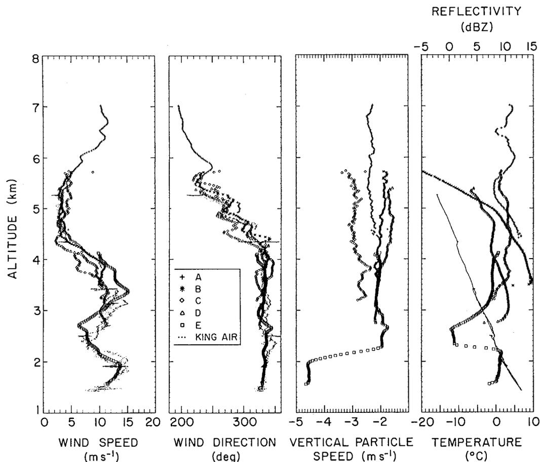
FIG. 6. Wind profiles derived from KingAir data (dots) and AVAD analysis: (a) wind speed, (b) wind direction, (c) vertical particle speed, and (d) temperature and mean reflectivity. Labels A–E on the profiles correspond to the similarly labeled data segments in Fig. 5.
