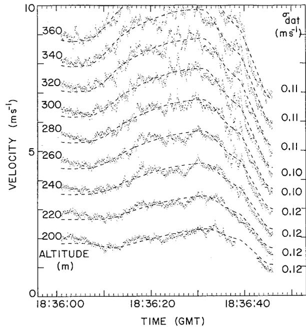
FIG. 3. Least squares fit (dashed line) and measured Doppler velocity (dots).
