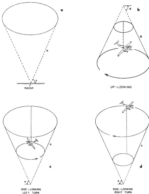
FIG. 1. Scanning geometry for (a) ground-based radar, (b) up-looking radar beam (left or right turn), (c) side-looking radar beam (left turn), and (d) side-looking radar beam (right turn).
