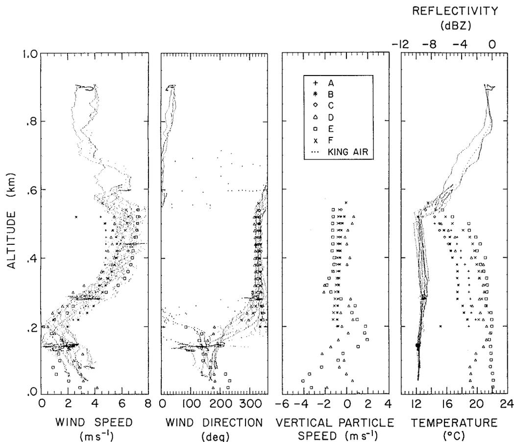
FIG. 8. Wind profiles derived from KingAir data (dots) and AVAD analysis: (a) wind speed, (b) wind direction, (c) vertical particle speed, and (d) temperature and mean reflectivity. Labels A–F on the profiles correspond to the similarly labeled data segments in Fig. 7.
