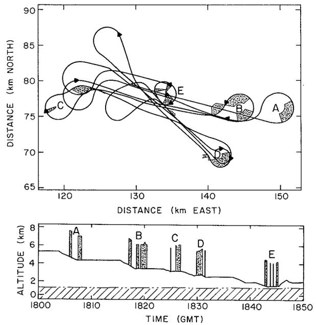
FIG. 5. (a) Map view of flight tracks and areas of coverage for the AVAD analyses. Labels A–E mark the locations of profiles. (b) Flight altitudes and times for the data used in the AVAD analyses. All profiles are up-looking.
