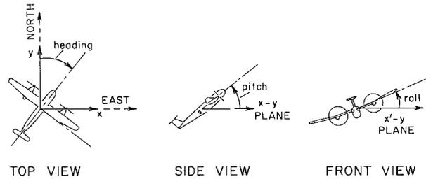
FIG. 2. Heading ( $\psi$ ), pitch ( $\theta$ ), and roll ( $\phi$ ) angles [adapted from Lenschow (1971)].
