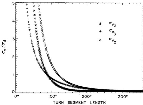
FIG. 4. Standard deviation of the velocity component estimates as a function of the length of the turn segment used. One independent Doppler velocity sample per degree is assumed along with an effective elevation angle of 30° and with the beam initially pointing to the east.
