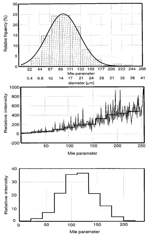
FIG. 2. (a) Typical observed droplet spectrum. (b) Intensity of the Mie scattering at  $90^\circ$  in the function of the Mie parameter calculated with a 2-m resolution and averaged on bins as in (a). (c) Effect of the droplet spectra on the intensity of scattered light at a  $90^\circ$  angle.
