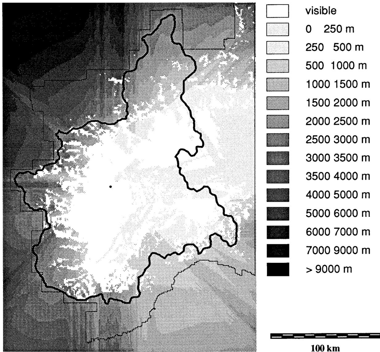
FIG. 6. Minimum height (MSL) that a meteorological target must reach to be optically seen from the radar site ( $R_{\text{eq}}/R_{\text{earth}} = 1.34$ ).
