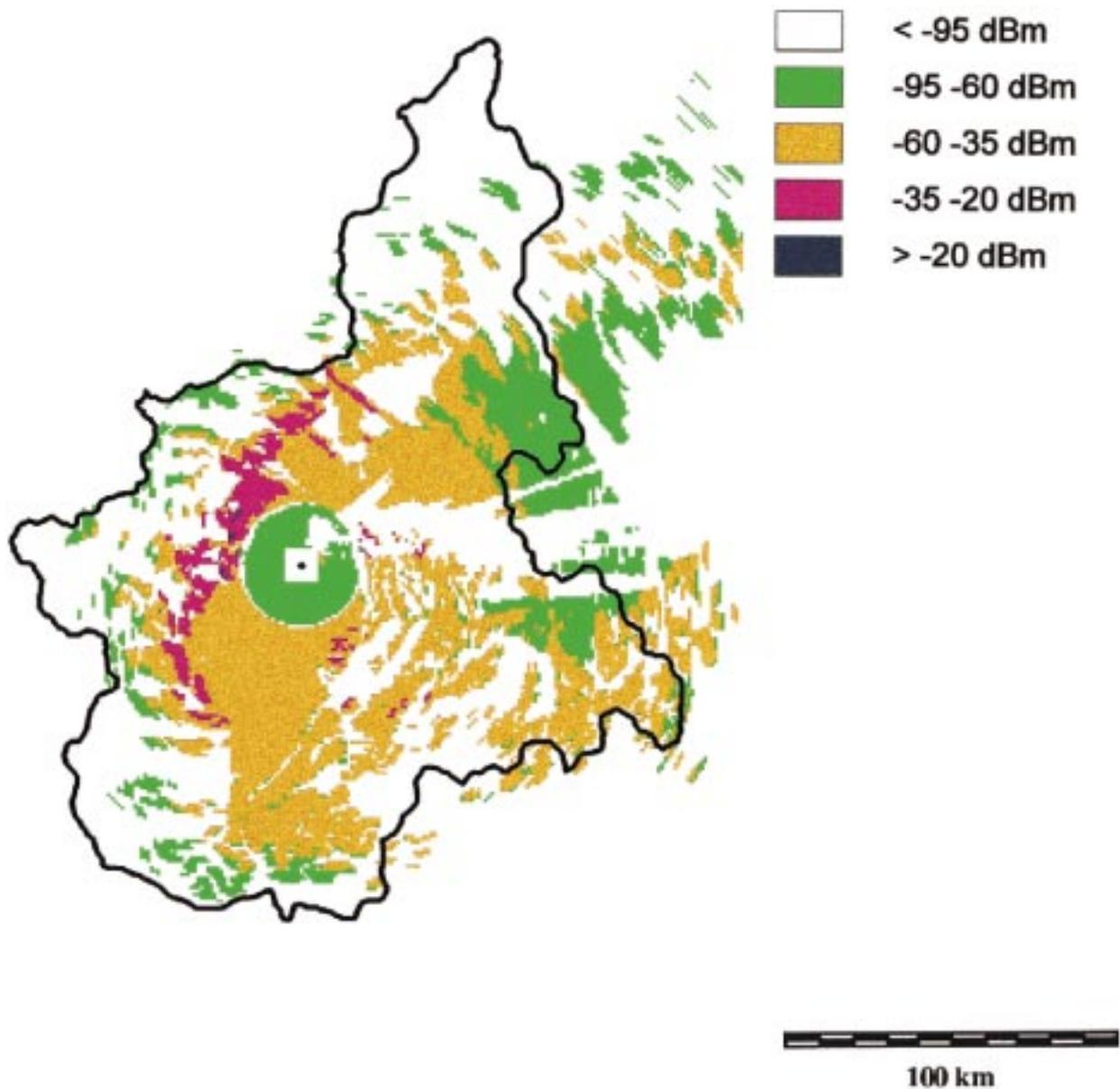
FIG. 7. Simulated ground clutter in clear-sky, dry weather condition ( $R_{\text{eq}}/R_{\text{earth}} = 1.34$ ).
