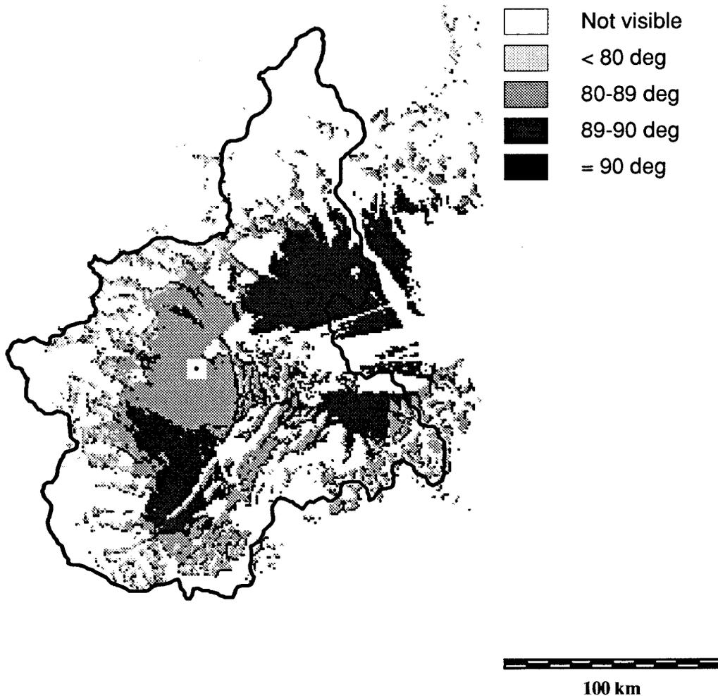
FIG. 4. Angles of incidence map ( $R_{eq}/R_{earth} = 1.34$ ). The white  $10 \text{ km} \times 10 \text{ km}$  square area centered around the radar site (black circle) is the zone where no data are acquired.
