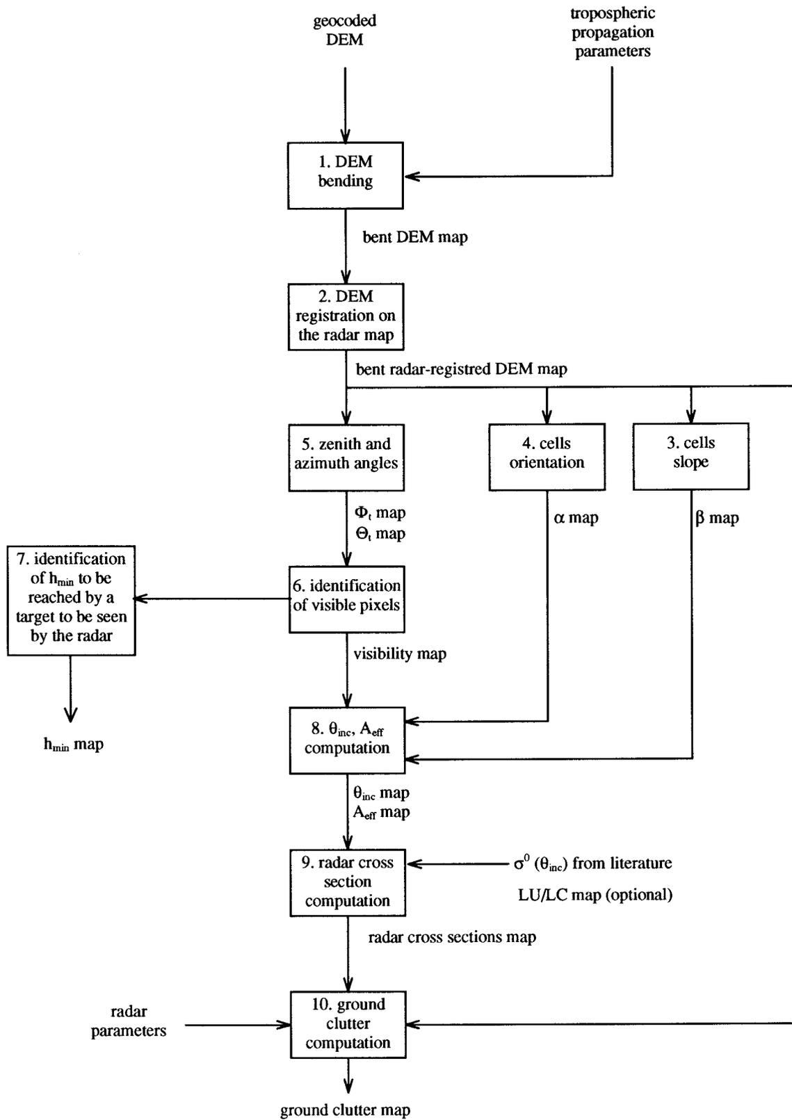
FIG. 1. Ground echo characterization software flowchart.
