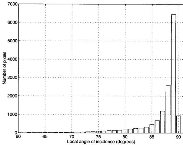
FIG. 5. Histogram of the angles of incidence map represented in Fig. 4 with 1° resolution (mean value = 87°, median value = 89°, standard deviation = 3.7°, and interquartile range = 2° centered at 88°).
