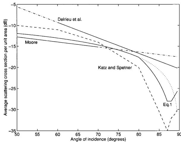
FIG. 2. Average scattering cross section per unit area,  $\bar{\sigma}_{\text{dB}}^0$ , at large angles of incidence.
