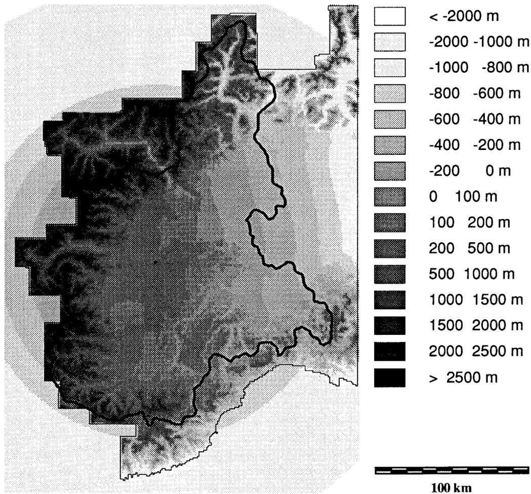
FIG. 3. Bent and resampled DEM registered on the radar Cartesian map (known atmospheric refractivity profile:  $R_{\text{eq}}/R_{\text{earth}} = 1.34$ ).
