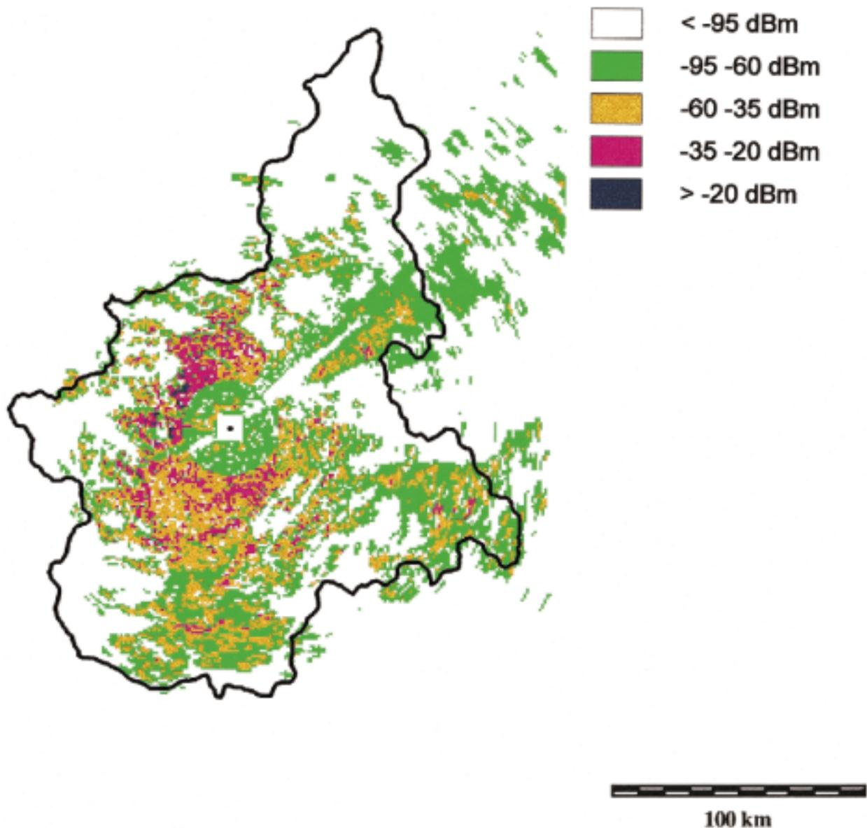
FIG. 8. Ground clutter power measured by the radar situation at 1100 UTC 6 December 1994 (clear-sky, dry weather condition and quasi-constant value of atmospheric refractivity profile:  $R_{\text{eq}}/R_{\text{earth}} = 1.34$ ).
