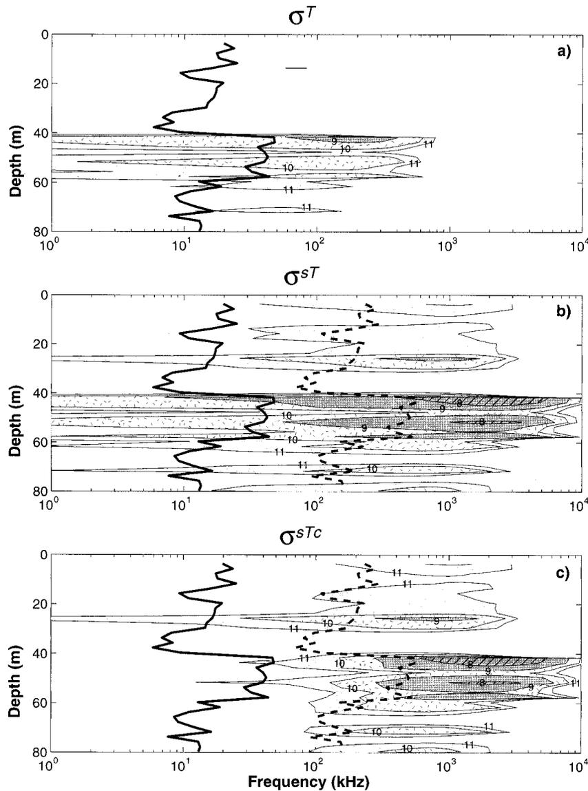
FIG. 5. Contours of  $\sigma$  as a function of depth and acoustic frequency for Admiralty Inlet in Puget Sound. Panels are as in Fig. 3. Including salinity greatly increases  $\sigma$  at all frequencies. The cospectrum strongly suppresses  $\sigma$  below  $f(k_{\text{int}})$  because  $R_\eta \approx -1$ , leaving large  $\sigma$  only above 100 kHz.
