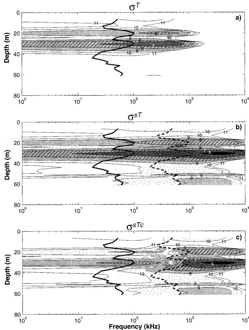
FIG. 4. Contours of  $\sigma$  as a function of depth and acoustic frequency for the Bosphorus. Panels are as in Fig. 3. Small  $\delta$  causes the inclusion of salinity to dramatically alter  $\sigma$ . The cospectrum introduces deep, narrow notches near  $f(k_d)$ , where  $R_\eta \approx -1.5$ .
