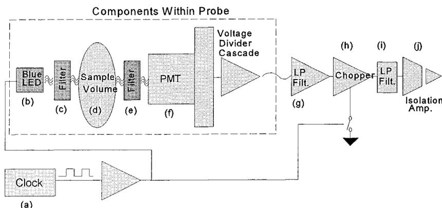
FIG. 1. Schematic of overall fluorometer design.
