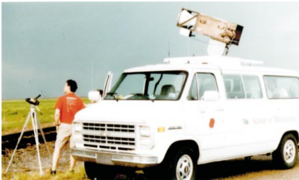
FIG. 3. The 95-GHz polarimetric cloud radar and chase van during a measurement.
