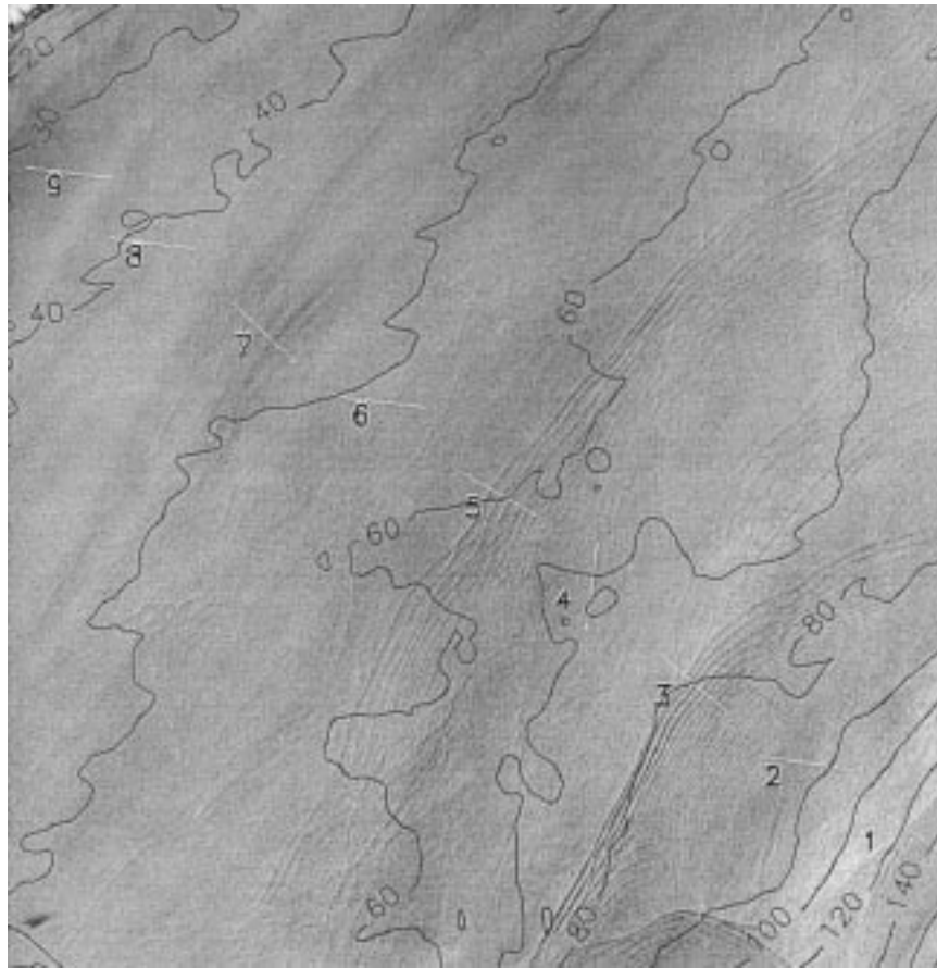
FIG. 10. Image showing the wave direction computed using the Radon method.
