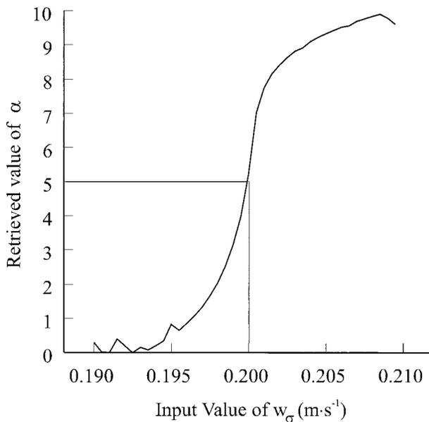
FIG. 2. The retrieved value of the shape parameter ( $\alpha$ ) as a function of the turbulent intensity ( $w_\sigma$ ) during the phase II fitting process. The curve was constructed using simulated spectral data and the correct value of  $w_M$ . Correct values of  $\alpha$  and  $w_\sigma$  are indicated by reference lines.
