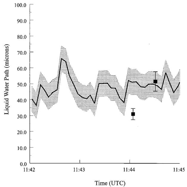
FIG. 11. Comparison of total liquid water path from a microwave radiometer (solid line) and retrieved profiles. Symbols (■) indicate mean retrieved values and error bars show retrieval uncertainties. The shaded area denotes the radiometer’s random instrument error.
