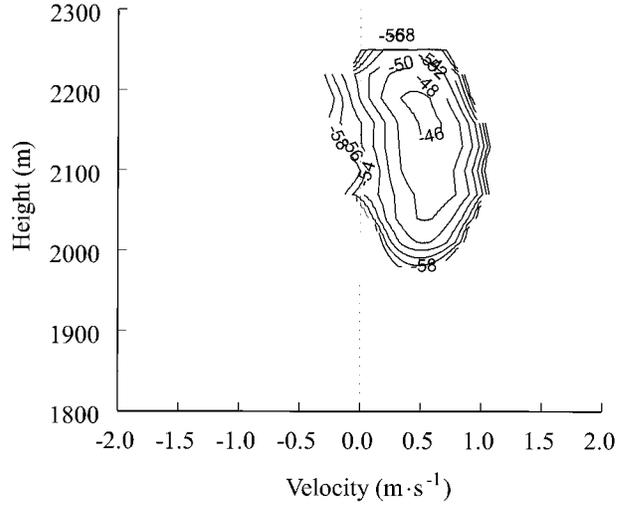
FIG. 6. A spectrograph taken from a nonprecipitating region of the cloud. Contour lines are levels of spectral reflectivity with units  $10 \log_{10} [\text{mm}^6 \text{m}^{-3} (\text{m s}^{-1})^{-1}]$ .
