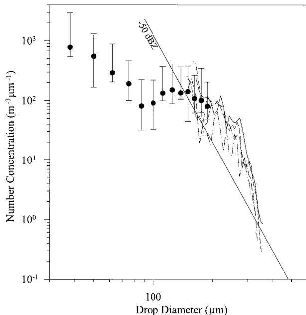
FIG. 12. Retrievals of the precipitation portion of the drop distribution (various lines). For comparison aircraft observations obtained from a 1-DC probe are also shown. Error bars denote maximum and minimum 1-DC concentrations with symbols indicating the mean concentrations. Also shown is the  $-50$ -dBZ contour as a function of the two axes, which represents the approximate maximum spectral sensitivity of the radar at 2 km.
