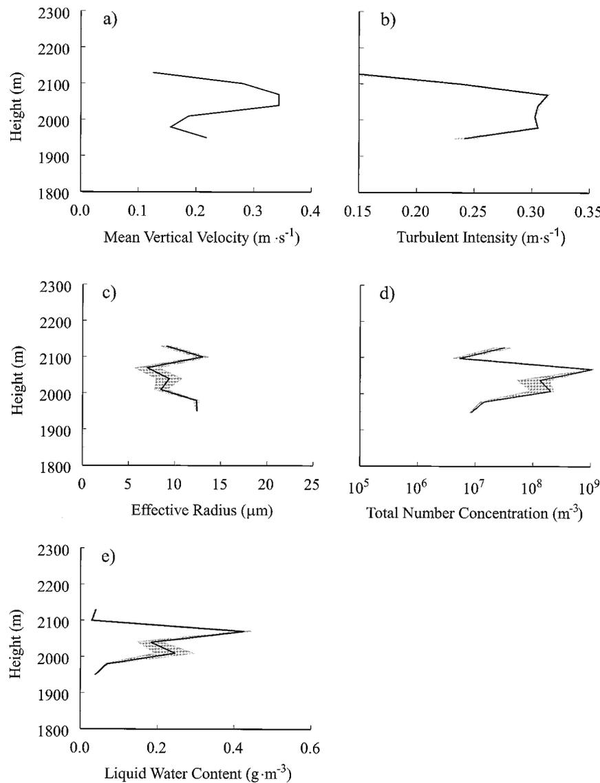
FIG. 8. Profiles of (a) mean vertical wind and (b) retrieved  $w_{\sigma}$  for 1144:04 UTC. Also shown are profiles of (c) effective radius, (d) total number concentration, and (e) LWC calculated from the retrieved parameters. For each profile, the solid line represents the mean retrieved solution and the shading indicates retrieval uncertainty.
