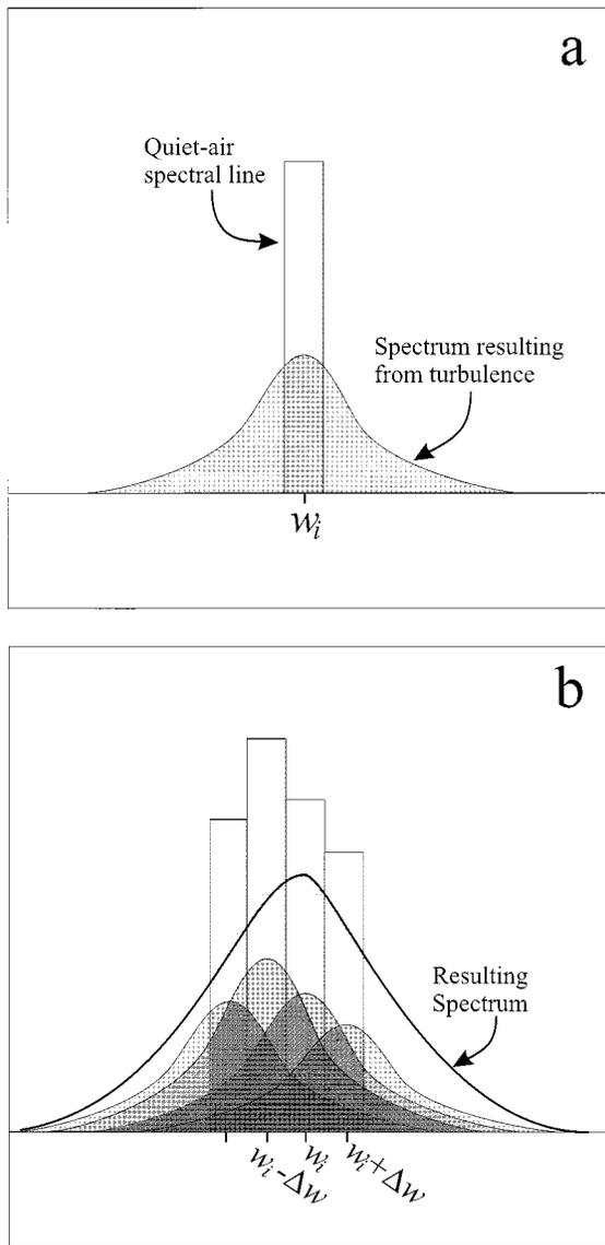
FIG. 1. Representation of the effect of turbulent broadening (a) on a single spectral line and (b) on a spectrum consisting of several spectral lines.
