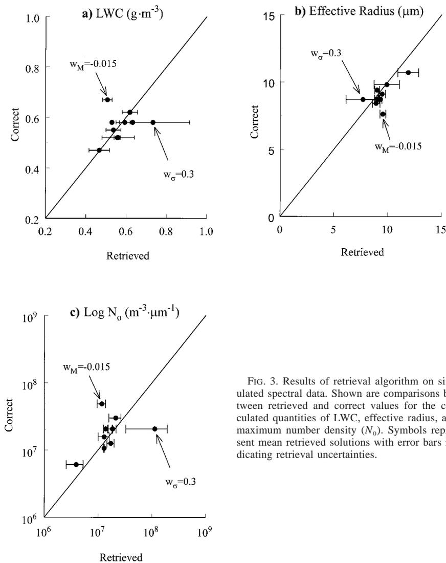
FIG. 3. Results of retrieval algorithm on simulated spectral data. Shown are comparisons between retrieved and correct values for the calculated quantities of LWC, effective radius, and maximum number density ( $N_0$ ). Symbols represent mean retrieved solutions with error bars indicating retrieval uncertainties.
