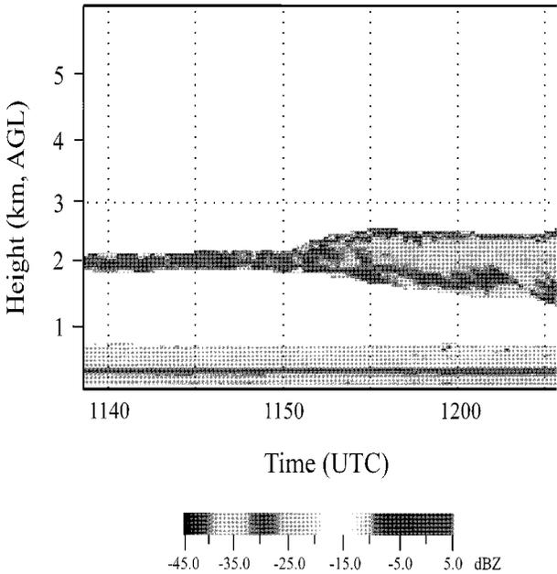
FIG. 5. Time–height profile of integrated reflectivity constructed from the vertically pointing 94-GHz radar.
