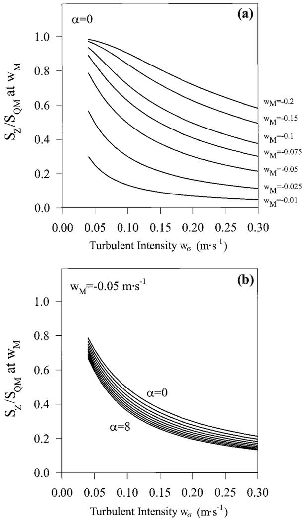
FIG. 13. Graphs showing the effects of turbulent broadening as a function of (a)  $w_M$  and (b)  $\alpha$ . The ratio  $S_z/S_{QM}$  at  $w_M$  is a measure of how much the quiet-air peak has been reduced as a result of turbulence.
