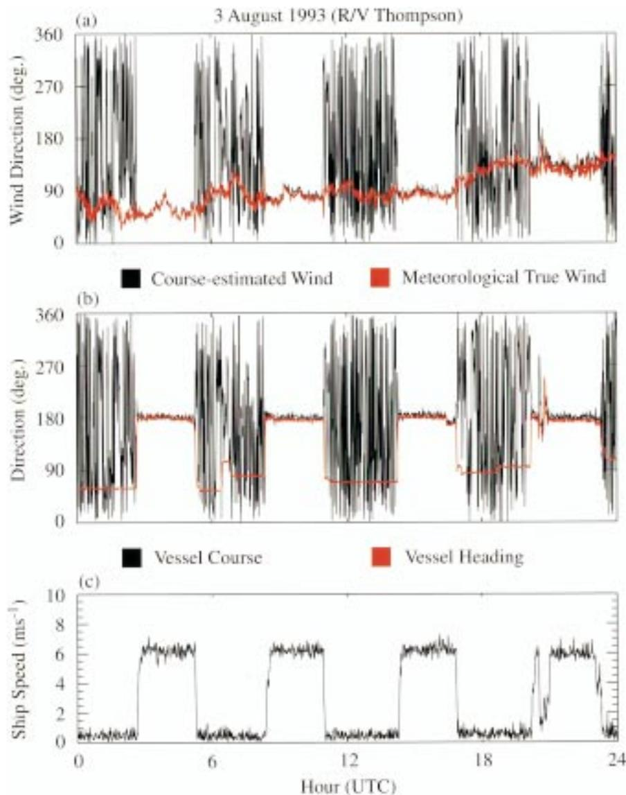
FIG. 3. Time series plots of (a) course-estimated (black) vs meteorological true (red) wind direction, (b) vessel course (black) vs heading (red), and (c) vessel speed over the ground from the R/V *Thompson* (3 Aug 1993).
