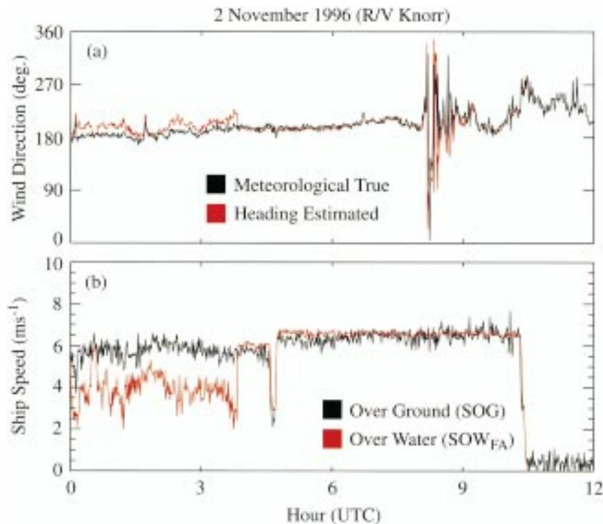
FIG. 5. Time series plots of (a) heading-estimated (red) vs meteorological true (black) wind direction and (b) vessel speed over the water (red) vs the speed over the ground (black) from the R/V *Knorr* (2 Nov 1996). Note that the speed over the water drops out after 1030 UTC due to an instrument malfunction.
