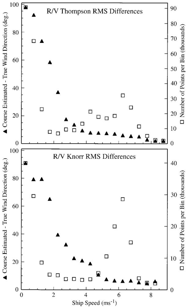
FIG. 4. Rms differences of course-estimated minus true wind direction (filled triangles) from the R/V *Thompson* and R/V *Knorr*. Rms differences are calculated for 0.5 m s<sup>-1</sup> bins of the vessel's speed over the ground using the absolute value of the wind direction differences (i.e., range 0°–180°). The number of values in each bin (open squares) are presented in units of thousands.
