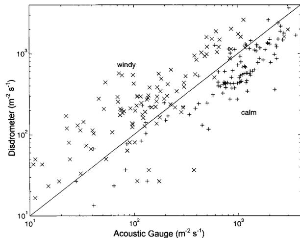
FIG. 15. The influence of wind on the small drop population estimates by the acoustic inversion and the disdrometer. The acoustic small populations estimates during calm conditions,  $U < 2$   $\text{m s}^{-1}$ , “+” symbols, are higher by a factor of 3 than during windy conditions,  $U > 5$   $\text{m s}^{-1}$ , the “x” symbols.
