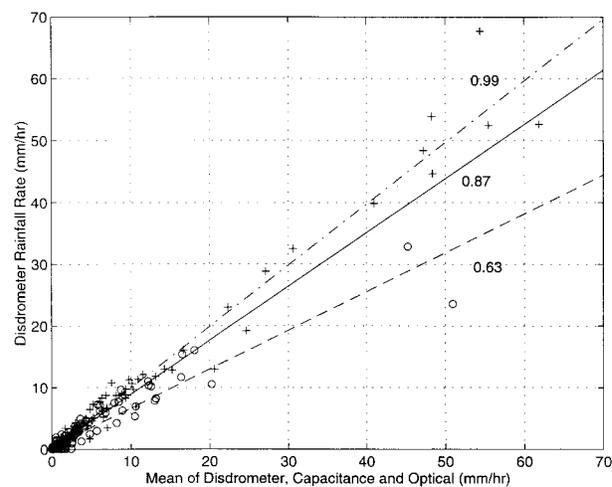
FIG. 8. Disdrometer rainfall rates compared to the mean of the disdrometer, capacitance and optical rain gauges for different wind speeds during TS Gordon. Three categories are shown: calm, <2 m s<sup>-1</sup>, “+” symbol, dash-dot line; breezy, 2–5 m s<sup>-1</sup>, solid line; and windy, >5 m s<sup>-1</sup>, “o” symbol, dashed line. Individual data points for the breezy category are not shown. The slope of the first order regression is indicated next to each regression line.
