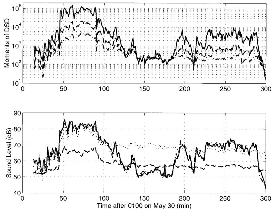
FIG. 5. Measured moments of the drop size distribution (upper panel) from the disdrometer. Shown are  $M_2$  (solid line),  $M_4$  (dashed line), and  $M_6$  (solid line). The units are mm <sup>$x$</sup>  m<sup>-3</sup>, where  $x$  is the moment (2nd, 4th, or 6th). The bottom panel shows the sound level at four selected frequencies: 2 kHz (solid), 5 kHz (dash-dot), 15 kHz (dotted), and 40 kHz (dashed). The units are dB relative to 1  $\mu$ Pa<sup>2</sup> Hz<sup>-1</sup>.
