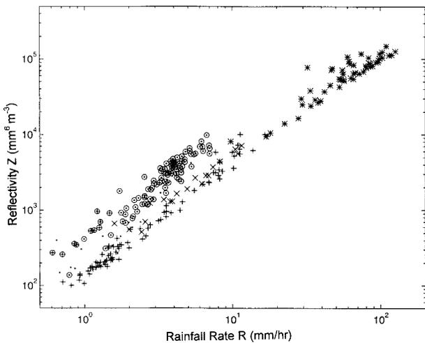
FIG. 4. The  $Z$ - $R$  (reflectivity-rainfall rate) relationship for event 150 at 0113 (30 May 1994). Different periods of the event are marked with different symbols: Mins 13-24 “ $\oplus$ ”; Mins 25-44 “ $\times$ ”; Mins 45-100 “ $*$ ”; Mins 101-180 “ $+$ ” and Mins 200-300 “ $\odot$ .”
