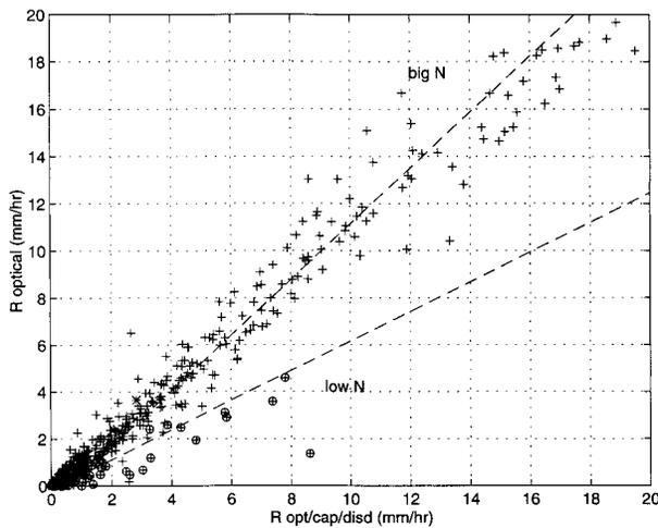
FIG. 11. Optical rain gauge performance as a function of  $N_0$ . The slope of the first-order regression is proportional to  $N_0$ . In this example, low  $N_0$  values ( $N_0 < 10^3$ ) are shown by the “⊕” symbols and dashed line (slope = 0.61) and high  $N_0$  values ( $N_0 > 10^4$ ) are shown by the “+” symbols and solid line (slope = 1.06). Intermediate data points ( $10^3 < N_0 < 10^4$ ) are not shown.
