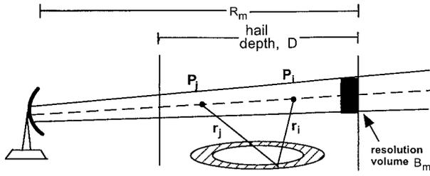
FIG. 2. A schematic of three-body scattering. Signal path: radar  $\rightarrow$  particle  $P_i \rightarrow$  ground  $\rightarrow$  particle  $P_j \rightarrow$  radar. The hatched area represents the area on the ground where the three-body path has the same time delay as the direct path from the radar to the resolution volume  $B_m$ .
