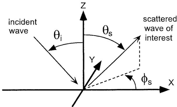
FIG. 3. The three-body scattering geometry for a ground element. Incident wave direction is always in the  $x$ - $z$  plane.
