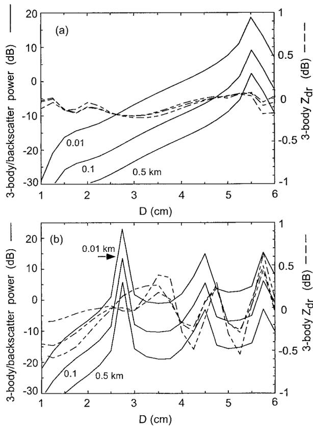
FIG. 9. The ratio of three-body scatter power to direct backscatter power (left axis) and three-body  $Z_{DR}$  as a function of hail diameter. Spherical hail is modeled as an ice core with a liquid water coat (1 mm). The Lommel–Seeliger ground model is used at (a) S band and (b) C band.
