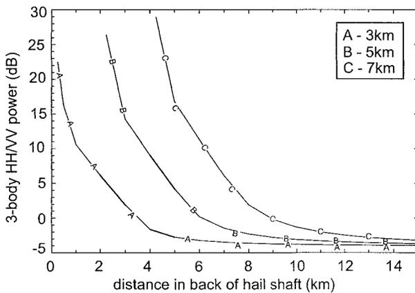
FIG. 8. The three-body power ratio HH/VV as a function of distance in back of the hailshaft.
