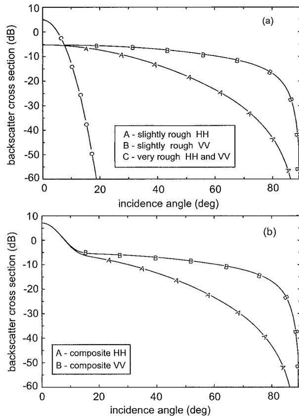
FIG. 5. The backscatter cross section ( $\theta_i = \theta_s$ ) for (a) the very rough and slightly rough surface models and (b) the composite model.
