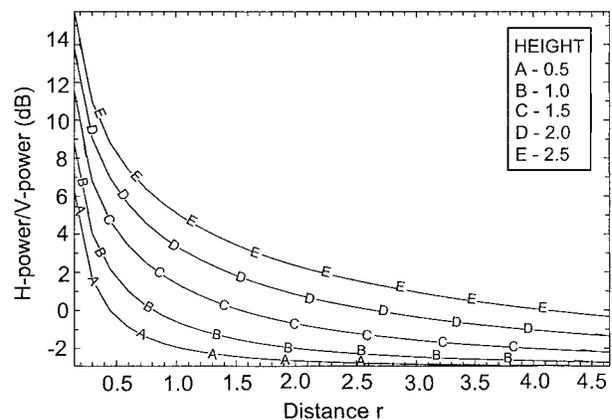
FIG. 7. The ratio of horizontal to vertical power incident on the hatched area in Fig. 6 with  $h$  as a parameter. The horizontal axis is in arbitrary units of  $r_i$  and  $r_{i+1} = 0.15 + r_i$ .
