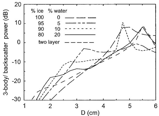
FIG. 11. The ratio of three-body scatter power to direct backscatter power for various mixtures of ice and water. Two-layer denotes water-coated ice spheres.
