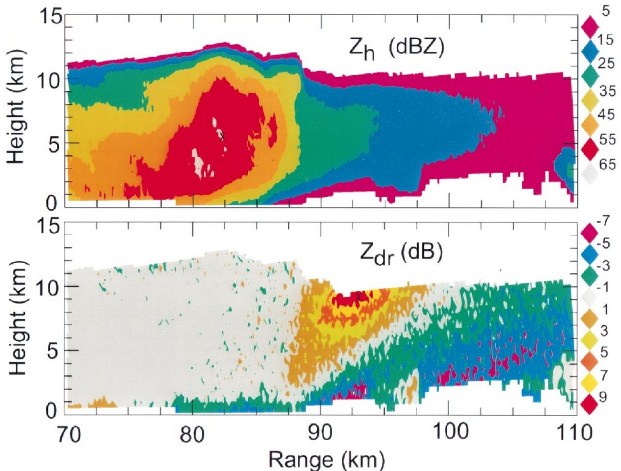
FIG. 1. An example of three-body scattering in a hailstorm from DLR's (German Aerospace Agency) C-band radar located at Oberpfaffenhofen, Germany. The three-body signature is easily seen as the protruding reflectivity area on the right-hand side in the top panel. The bottom panel shows the associated  $Z_{DR}$  (differential reflectivity).
