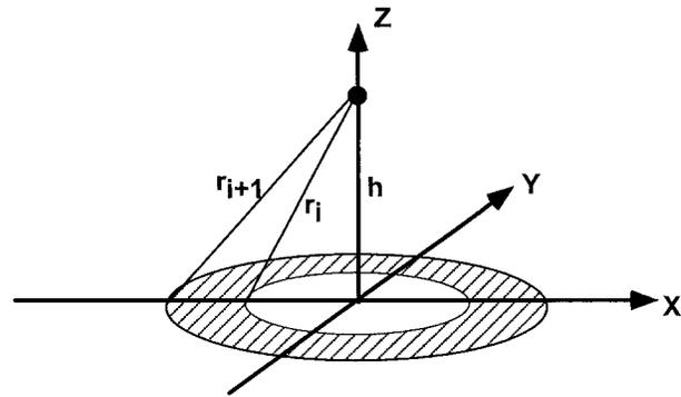
FIG. 6. Geometry for dipole field calculation. Dipole is located at height  $h$  above  $x$ - $y$  plane. Incident wave is along the positive  $x$  direction. The lengths  $r_i, r_{i+1}$  define an area between concentric circles over which power from the vertical and horizontal dipole fields are summed.
