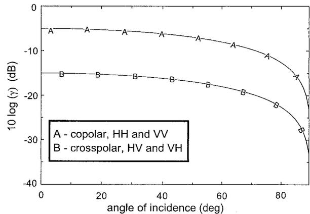
FIG. 4. The backscatter cross section  $\gamma$  for the Lommel–Seeliger model [Eq. (8)] for the ground. Note that  $\theta_i = \theta_s$  in Fig. 3.
