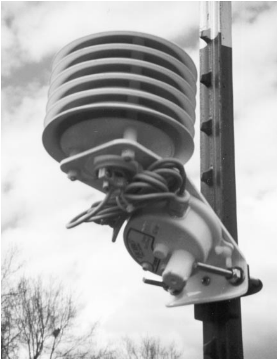
FIG. 1. Photograph of HOBO Pro Temp/Ext Temp datalogger and radiation shield mounted on a fence post. The round white plastic datalogger is mounted on the underside of the radiation shield mounting bracket; a 2-m electrical cable runs from the logger to a thermistor that is placed inside the radiation shield. A threaded plug at the end of a cylindrical projection from the face of the datalogger is removed to gain access to the logger for uploading instructions and downloading data.
