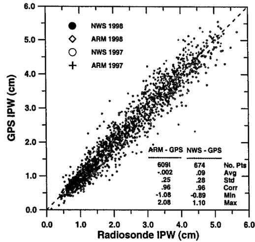
FIG. 14. ARM (PRCO) and NWS (Norman, OK) radiosonde IPW vs GPS-IPW (PRCO) scatterplot 1997-98. Statistics for 1997 only.
