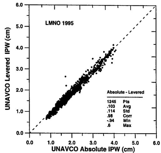
FIG. 6. UNAVCO-Bernese GPS absolute IPW vs levered IPW comparison: LMNO, 18 Apr-17 May 1995
