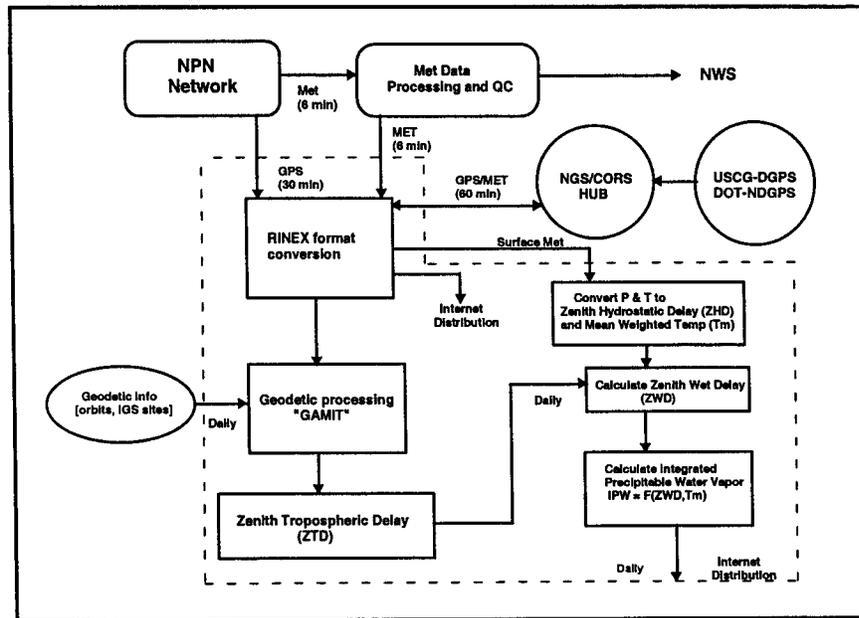
FIG. 11. GPS–IPW data flow–processing diagram. Region within the dotted line is controlled by the GPS Hub.
