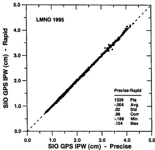
FIG. 4. Precise vs rapid orbit IPW comparison using SIO-GAMIT: LMNO, 18 Apr-17 May 1995.
