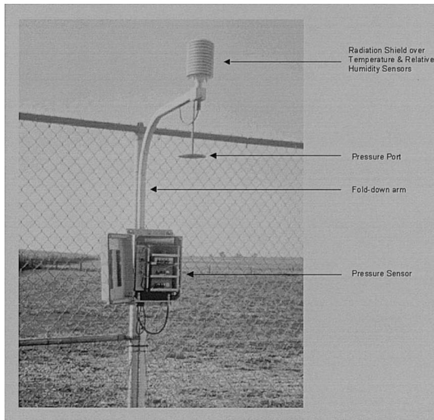
FIG. 12. GPS Surface Observing System: temperature, relative humidity, and pressure.
