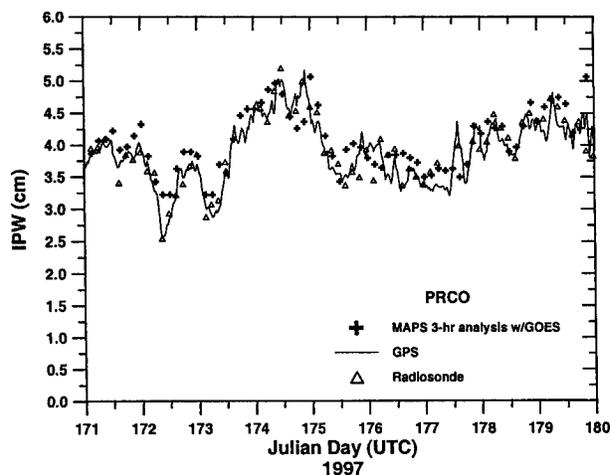
FIG. 10. MAPS 3-h analysis IPW, GPS-IPW, and ARM radiosonde IPW time series comparison: PRCO 1997.
