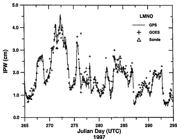
FIG. 9. GPS-IPW, GOES-IPW, and ARM radiosonde IPW time series comparison: LMNO 1997.
