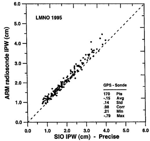
FIG. 5. SIO-GAMIT IPW using precise orbits vs radiosonde IPW: LMNO, 18 Apr-17 May 1995.
