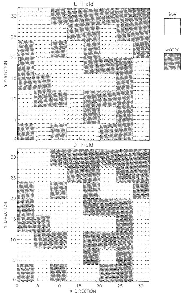
FIG. 1. Two-dimensional cut through a realization of a cubic particle composed of a water–ice mixture of equal fractional volumes. Arrows at each of the  $32 \times 32$  elements show the phasor representation of the  $x$  components of the  $\mathbf{E}$  and  $\mathbf{D}$  fields for an incident  $x$ -directed  $\mathbf{E}$  field propagating in the  $z$  direction. Minimum size of water and ice regions consists of  $4 \times 4 \times 4$  elements.
