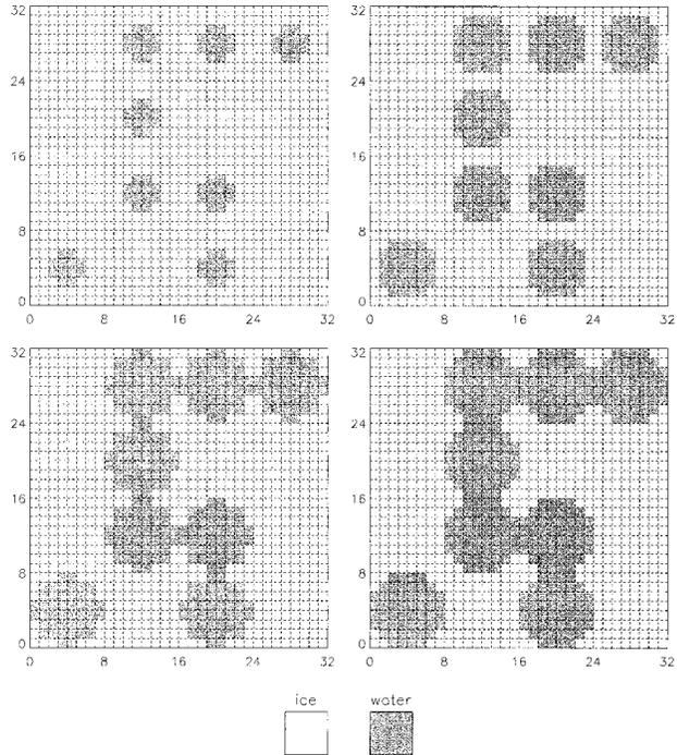
FIG. 9. Example of an ice–water particle mixture with water inclusions, of fractional volume 0.3, that are approximately spherical. The regions of water and ice are shown on four successive  $z =$  constant planes, where the difference in  $z$  from one cut to the next is equal to one element of the grid.
