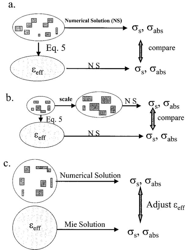
FIG. 10. Schematics of three procedures for checking the accuracy of  $\epsilon_{\text{eff}}$ .
