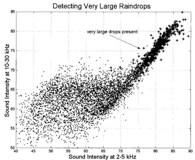
FIG. 5. A comparison of sound intensity at 2–5 and 10–30 kHz. The detection of very large raindrops in the rain can be achieved using these two frequency bands.
