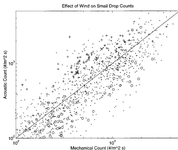
FIG. 11. The effect of wind on the small drop population count during TS Gordon (Nov 1994). During windy conditions ( $U > 5$  m  $s^{-1}$ , “O” symbol) the acoustic small drop count is a factor of 3 lower than during calm conditions ( $U < 2$  m  $s^{-1}$ , “+” symbol). Intermediate wind speed ( $2$  m  $s^{-1} < U < 5$  m  $s^{-1}$ ) points are shown by the “•” symbol.
