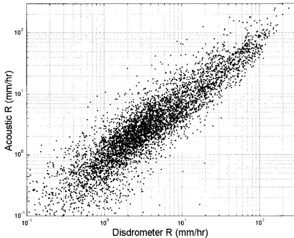
FIG. 8. Acoustic rainfall rate compared to disdrometer rainfall rate for over 6000 min of rainfall from Apr to Dec 1994. The correlation coefficient between the logarithms of the rainfall rate is  $r = 0.90$ .
