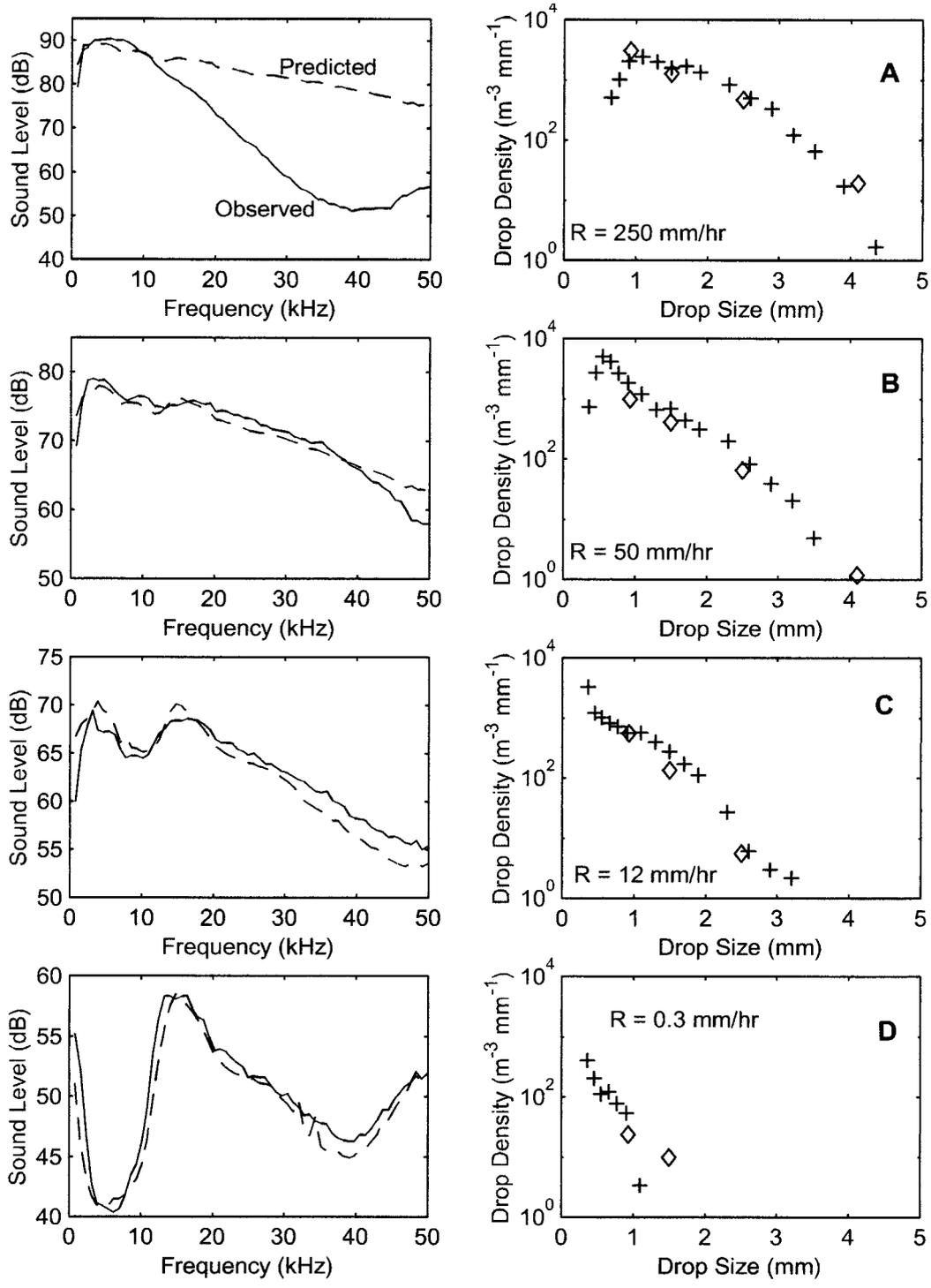
FIG. 6. Four examples of individual inversions to obtain drop size distribution. (right) The disdrometer data are shown, “+,” with the acoustic inversion results “◇.” (left) The observed sound field (solid line) is compared to the sound field predicted from the disdrometer data using the transfer function shown in Fig. 4 (the “forward problem”). Details for these four datasets (IDs = 114\_33, 256\_39, 256\_50, and 256\_68, respectively) are given in Table 1.
