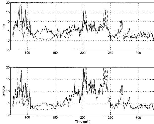
FIG. 15. The gamma distribution [Eq. (2)] shape parameters calculated by the method of moments (Ulbrich 1983) using the disdrometer data (solid line) and the acoustic inversion (dashed line) for event 150 at 0113. There is general agreement, except during the extreme convection from min 110 to 150. This event is also shown in Figs. 2, 3, and 14.
