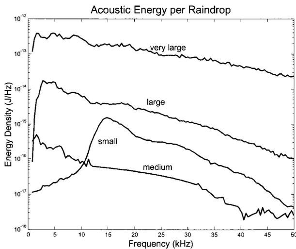
FIG. 4. The acoustic signature of individual drop size categories. This forms the basis for the inversion of the sound field to obtain drop size distribution.
