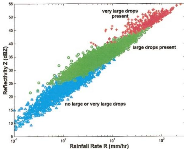
FIG. 13. The  $Z$ - $R$  relationship calculated from the JW disdrometer data and partitioned by acoustic inversion choice (Table 3). Each acoustic partition is associated with the presence or absence of particular drop sizes within the rain. Very large drops are present “+”; large drops are present, but no very large drops “O”; no large or very large drops “ $\Delta$ .”
