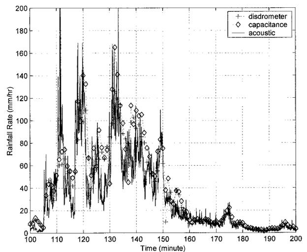
FIG. 17. High temporal resolution of the onset of the extreme convection during event 150 at 0113. The acoustic inversion has been applied with 5-s resolution (solid line) and shows rapid onset and cessation of subcells with the rain. Other rain gauge data shown with 1-min resolution are the disdrometer (+) and the capacitance gauge ( $\diamond$ ). This event is also depicted in Figs. 2, 3, 14, and 15.
