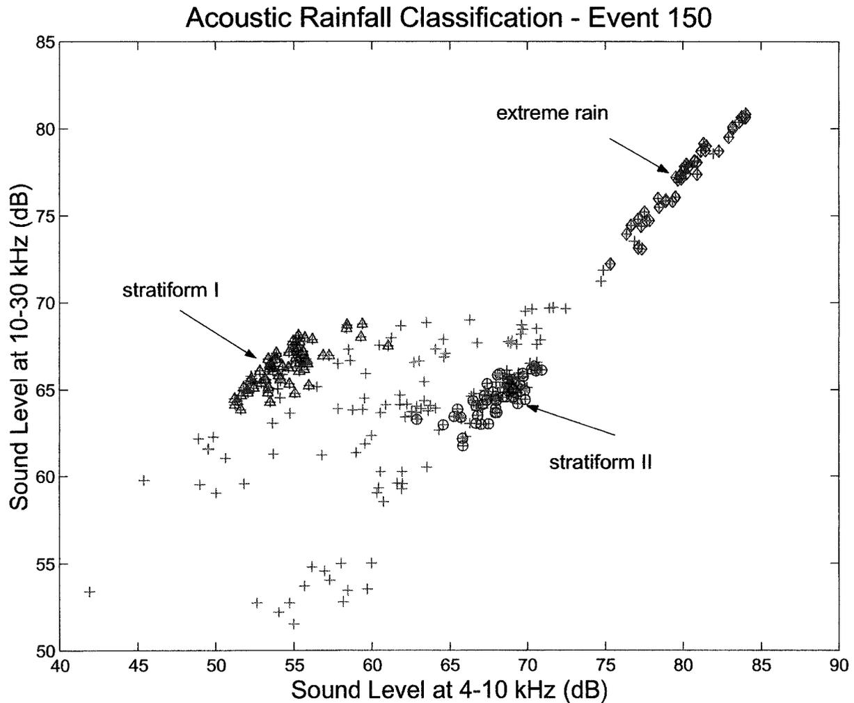
FIG. 14. The acoustic classification for event 150 at 0113. The data points for different rainfall types (extreme convection, stratiform I and II) are separated using a comparison of the sound levels at a lower frequency (4–10 kHz) and a higher frequency (10–30 kHz). This event is also shown in Figs. 2 and 3.
