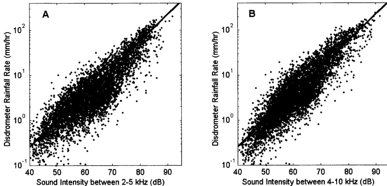
FIG. 12. The comparison of sound pressure levels and disdrometer derived rainfall rates for the frequency band 2–5 kHz (Fig. 12a) and 4–10 kHz (Fig. 12b). Equations (13) and (14) are shown for each dataset, respectively.
