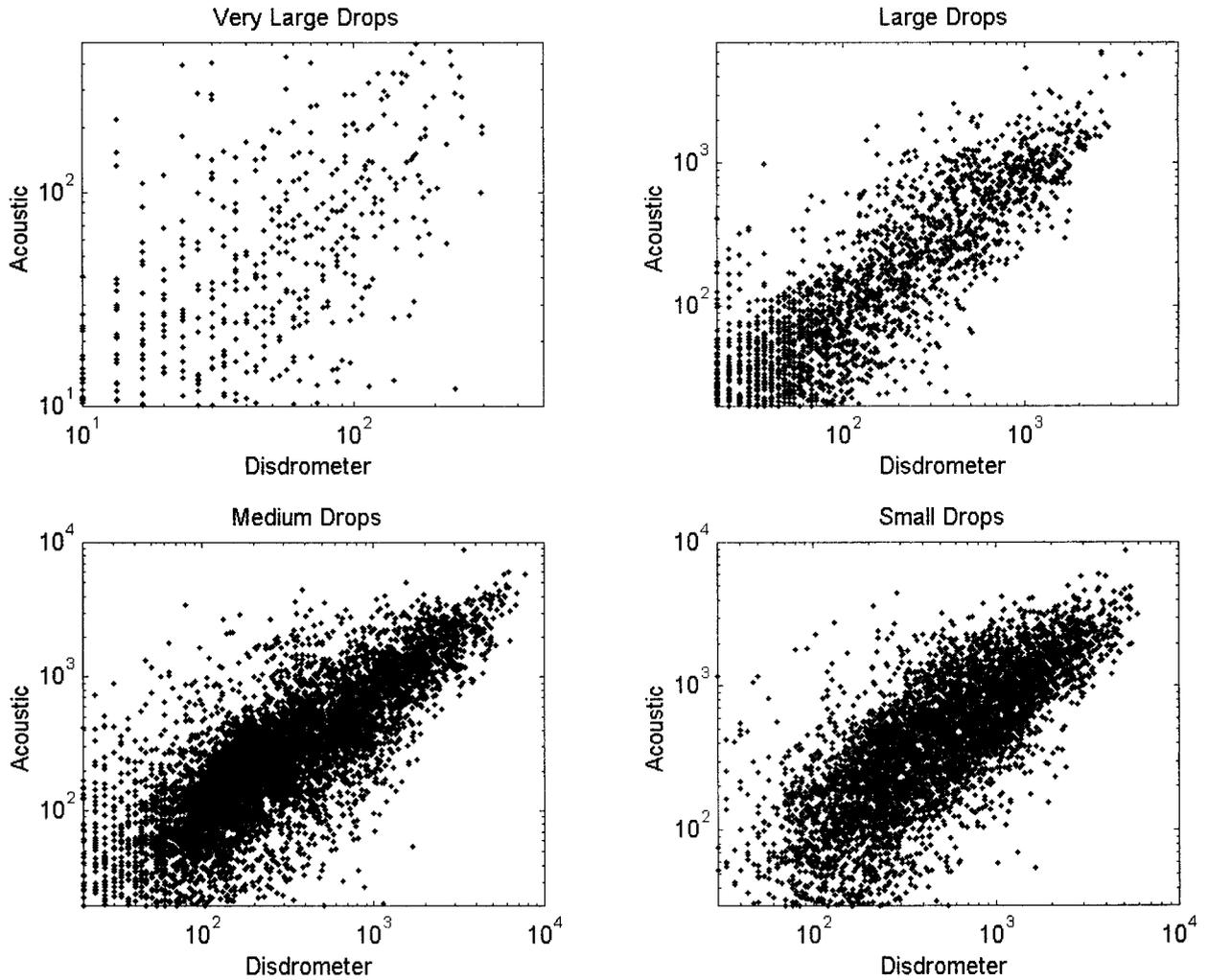
FIG. 7. The acoustic inversion drop count for each drop size category compared to the JW disdrometer drop count for the same drop size range. Data are from over 6000 min of rainfall from Apr to Dec 1994. The units are counts  $m^{-2} s^{-1}$ . The correlation coefficients for the logarithm of the counts are  $r = 0.56$  (very large drops),  $r = 0.86$  (large drops),  $r = 0.77$  (medium drops), and  $r = 0.76$  (small drops).
