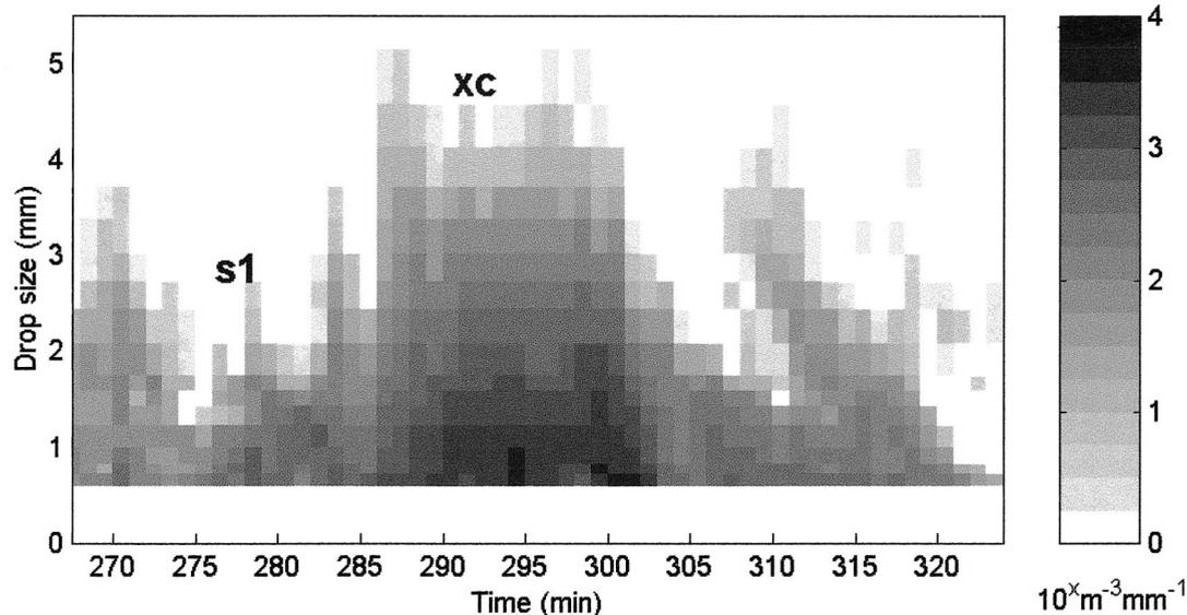
FIG. 10. An example of an unusual drop size distribution. The disdrometer shows a bimodal drop size distribution with relatively few medium-sized drops at min 310. The acoustic inversion overestimates the medium drop population leading to an overestimation in rainfall rate.
