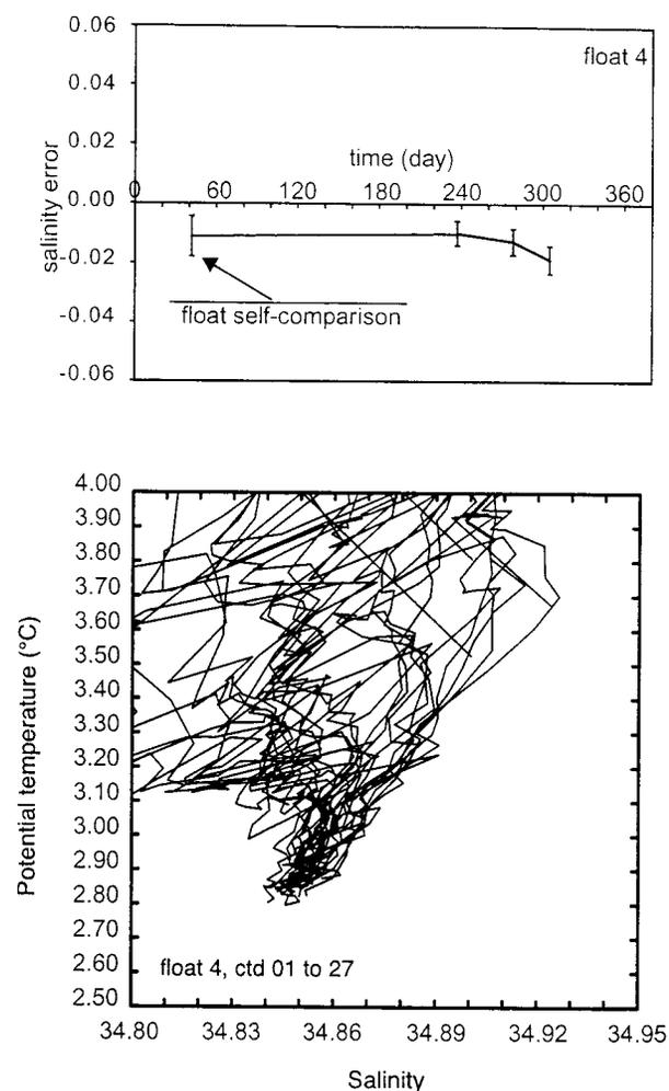
FIG. 8. A new calibration curve calculated by adding the offset computed by comparing the first and the second salinity profiles measured by the CTD package mounted on float 4 with (a) the fourth profile measured with the same instrument. (b) The  $\theta$ - $S$  diagram made with this new calibration curve. The spread of the envelope is reduced if compared with the similar diagrams shown in Fig. 6d.
