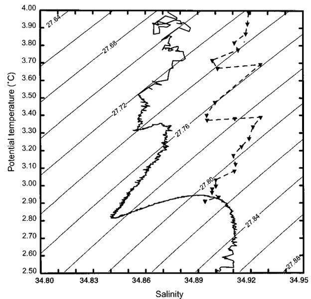
FIG. 4. Comparison, in  $\theta$ - $S$  space, of the uncorrected profile number 22 (2 Sep 1997) from float 3 with a ship CTD profile from *Discovery* cruise 230. The two stations are about 39 km apart. The ship CTD profile was made 24 h before the float profile. The two curves have similar slopes below 3.4°C and the salinity measured by the float appears to have an offset of  $\sim 0.04$ . Curves of constant  $\sigma_0$  are also superimposed.
