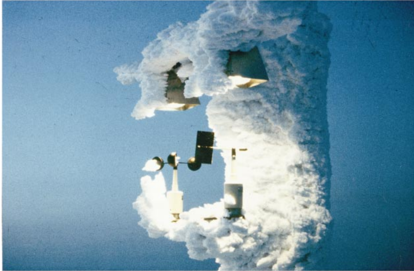
FIG. 1. Early attempt to anti-ice a cup anemometer using a 750-W infrared lamp. Photo is from 1983 at our test site on Yllas, Finland.
