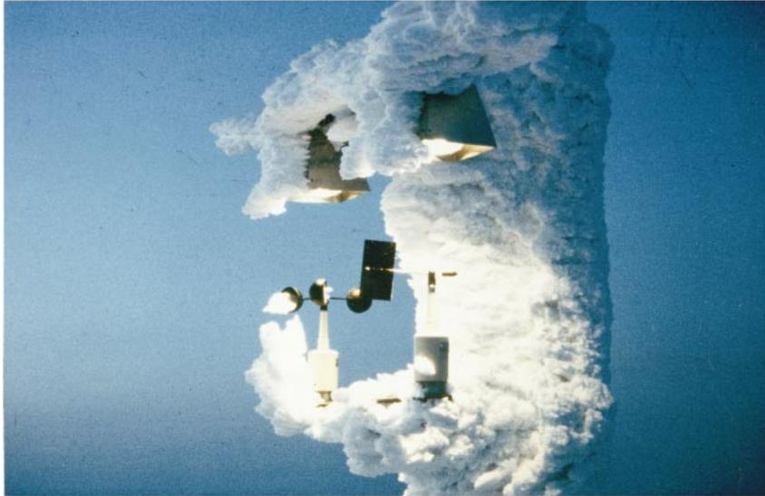
FIG. 1. Early attempt to anti-ice a cup anemometer using a 750-W infrared lamp. Photo is from 1983 at our test site on Yllas, Finland.
