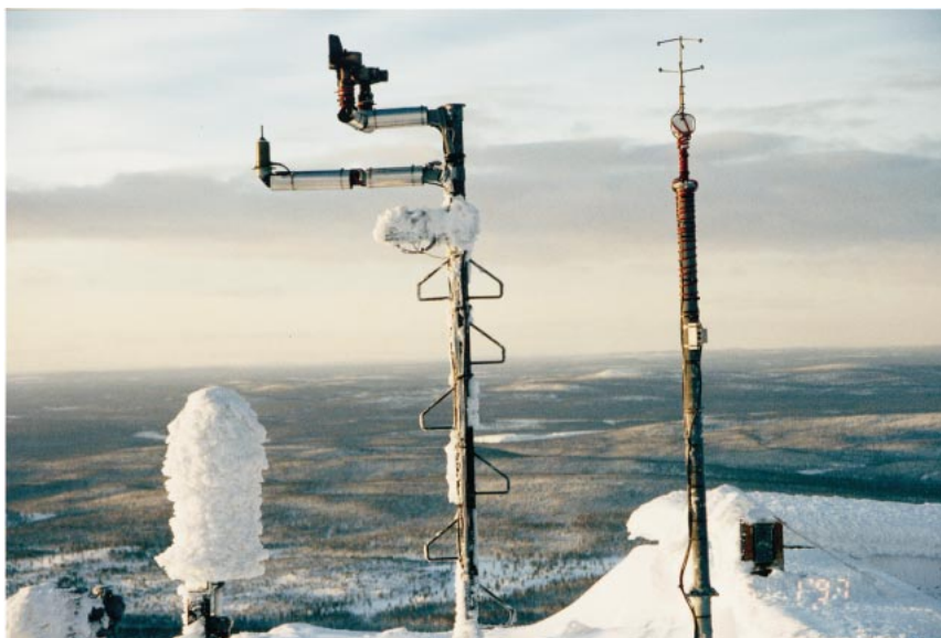
FIG. 6. Hydro-Tech (upper left) and Metek (separate support) anemometers at the field site. The supporting boom of the Hydro-Tech points to the south. The instrument on the other boom on the left is an Instrumar ice detector. The iced object at a lower level on the left is a 30-mm diameter cylinder used as an ice collector.
