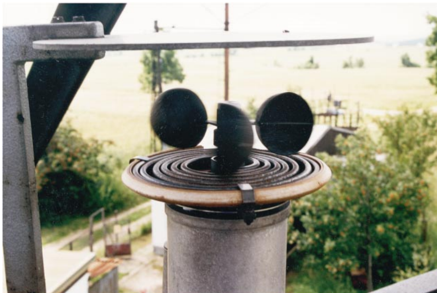
FIG. 2. Cup anemometer heated by a "frying pan" heater. Photo is from the icing research station in Studnice, Czech Republic.
