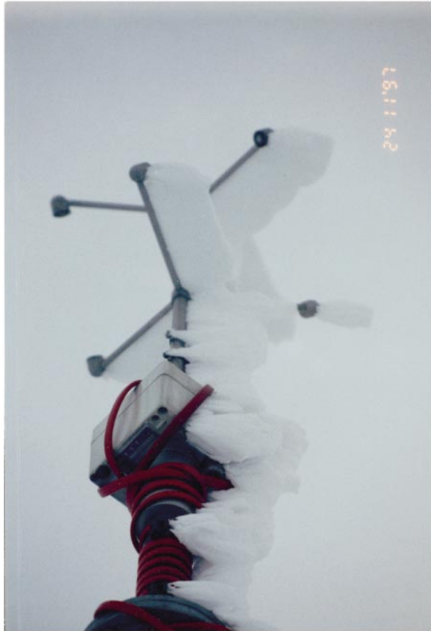
FIG. 7. Ice on a Metek sonic anemometer at the test site. This situation is atypical, but shows that sometimes icing of the instrument occurs in spite of the heating.
