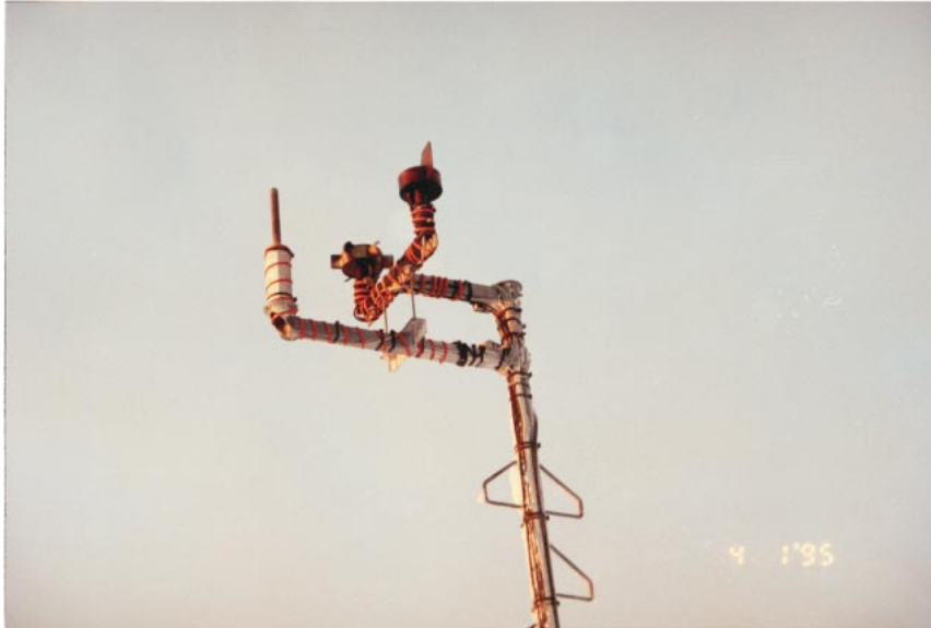
FIG. 5. Rosemount (left) and Hydro-Tech (right) anemometers at the field site. The supporting boom of the Rosemount is pointing to the south. Note the added heating cables to prevent icing of the supporting structures.
