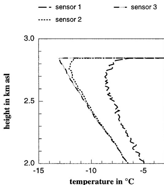
FIG. 2. Temperature profiles of sonde 2 with different sensor locations inside the duct close to (sensor 2) and far from the air inlet (sensor 1) as well as freely exposed about 10 cm outside (sensor 3).
