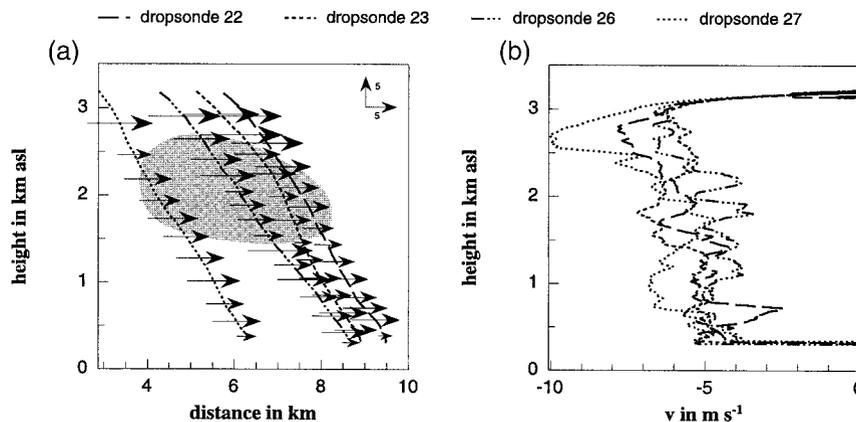
FIG. 4. Vertical structure of horizontal winds through a rapidly growing cumulus cloud derived from four dropsondes released at 3000 m within 52 s on 7 Jun 2000 near Karlsruhe. (a) The lines indicate the trajectories of the dropsondes in the  $x$ - $z$  plane. The  $x$  axis is parallel to the mean wind direction. The area of the cloud is shaded. (b) Falling speeds of the dropsondes as derived from the GPS heights.
