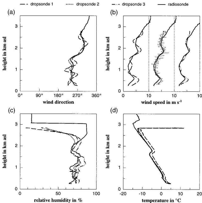
FIG. 3. Vertical profiles of (a) wind direction, (b) wind speed, (c) relative humidity, and (d) air temperature of three dropsondes and from a simultaneously launched AIR radiosonde. Wind speeds of the dropsondes are smoothed with a cutoff period of 60 s. The second diagram also includes the raw data (dotted).
