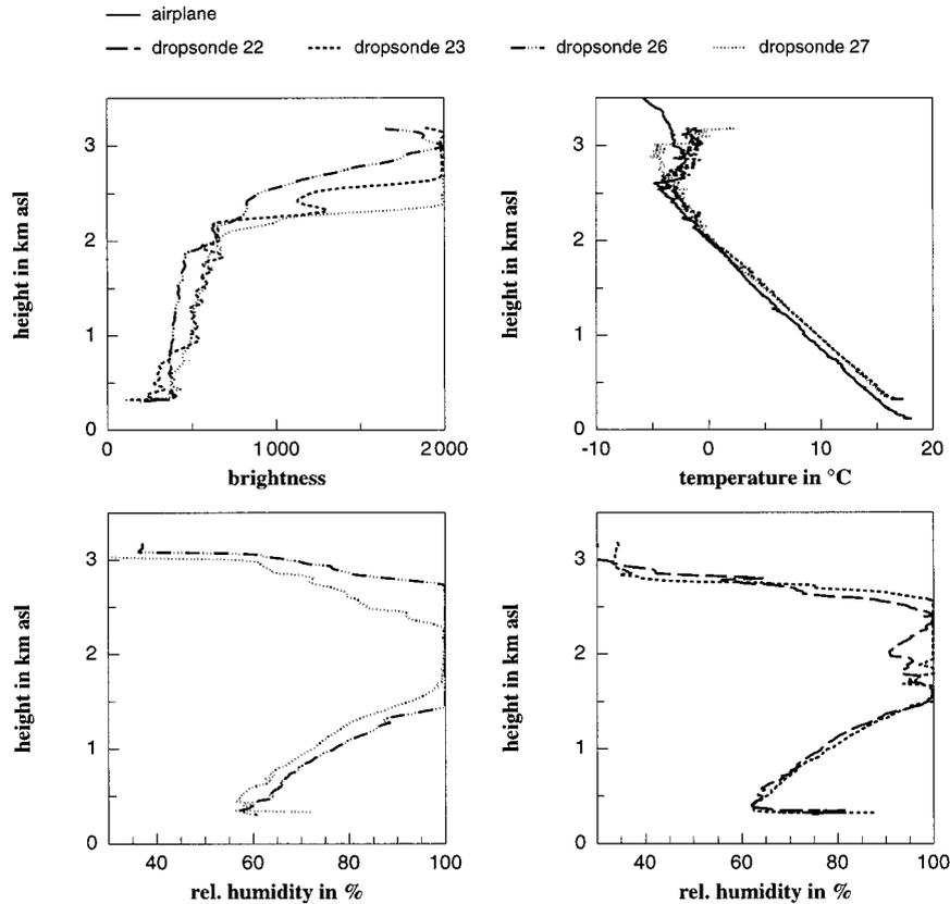
FIG. 5. Vertical profiles of relative humidity (bottom), temperature (upper right), and brightness (upper left) at different locations in the cumulus cloud. The locations of the dropsondes are given in Fig. 4. Additionally, the temperature profile measured by the aircraft between 1132 and 1149 LT is indicated.
