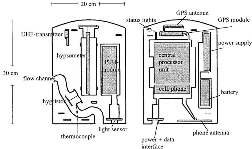
FIG. 1. Schematic overview of the dropsonde and its main components.
