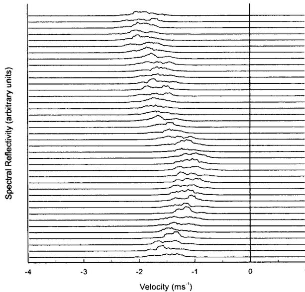
FIG. 2. Doppler power spectra derived from the cloud radar simulation model. Forty consecutive 512-point spectra are displayed, each with a small offset.
