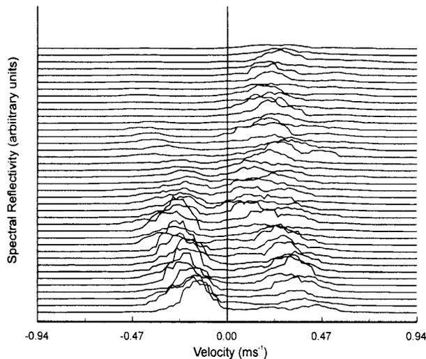
FIG. 8. Drizzle power spectra derived from the 12 Jun ASTEX stratocumulus dataset. Forty consecutive 512-point spectra are displayed, each with a small offset. Note the drizzle peak (toward faster fall velocities) fading away as the edge of a rain shaft moves away from the radar in the sampling period.
