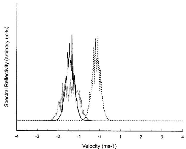
FIG. 4. Averaged Doppler power spectra for the simulated stratocumulus data. The three curves represent conventional incoherent average (gray), first moment-shifted average (black), and an average where the known vertical velocity values are removed (black, dotted), known as the optimal average.
