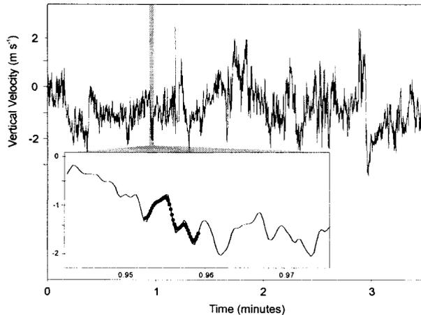
FIG. 1. Measurements of 50-Hz vertical velocity in continental stratocumulus. The inset shows the section of the data used in this study as input to the simulation. The 40 points on the subset curve represent the actual values selected for each spectral calculation. These points are representative of the volume sampled by the radar in 4 s under the assumption that there is a  $10 \text{ m s}^{-1}$  horizontal wind advecting the clouds over the radar site.
