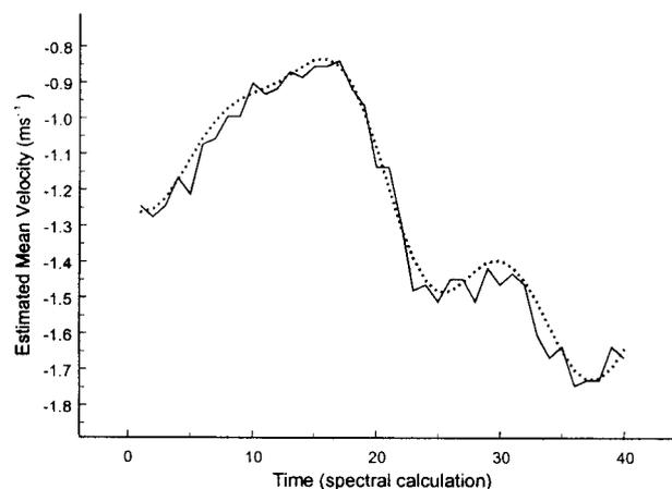
FIG. 5. Retrieved volume-mean vertical velocity field over the data sampling period (solid line) compared to the known vertical velocities of the simulated data (dotted line).
